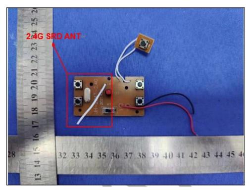
Length: 36mm Antenna Type: Wire Antenna Antenna Gain: 0dBi
