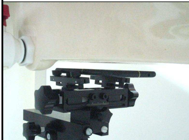
Front Face of EUT with 1.0 cm Gap
