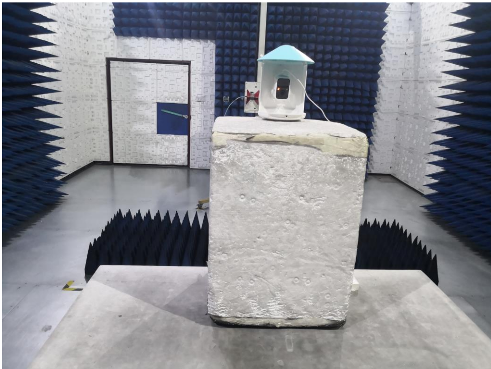
RADIATED EMISSION TEST SETUP ABOVE 1GHz
