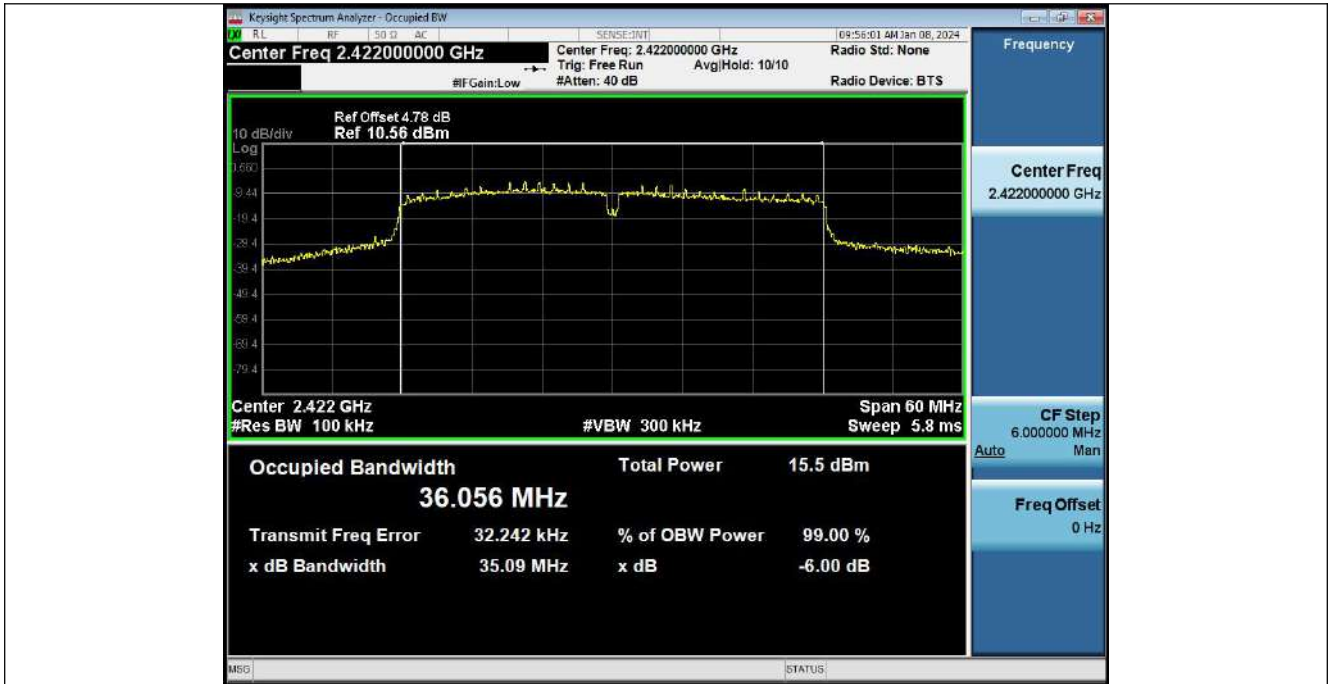
-6dB Bandwidth NVNT_ANT1_802_11n(HT40)_2437
