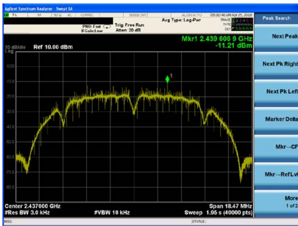
(802.11b) PSD plot on channel 11
