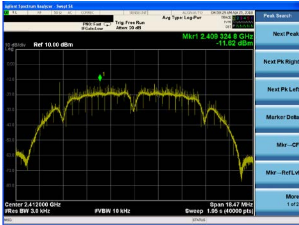
(802.11b) PSD plot on channel 6
