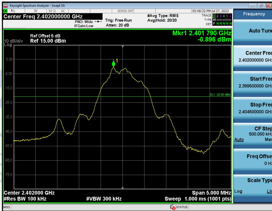
GFSK: Band Edge, Left Side
