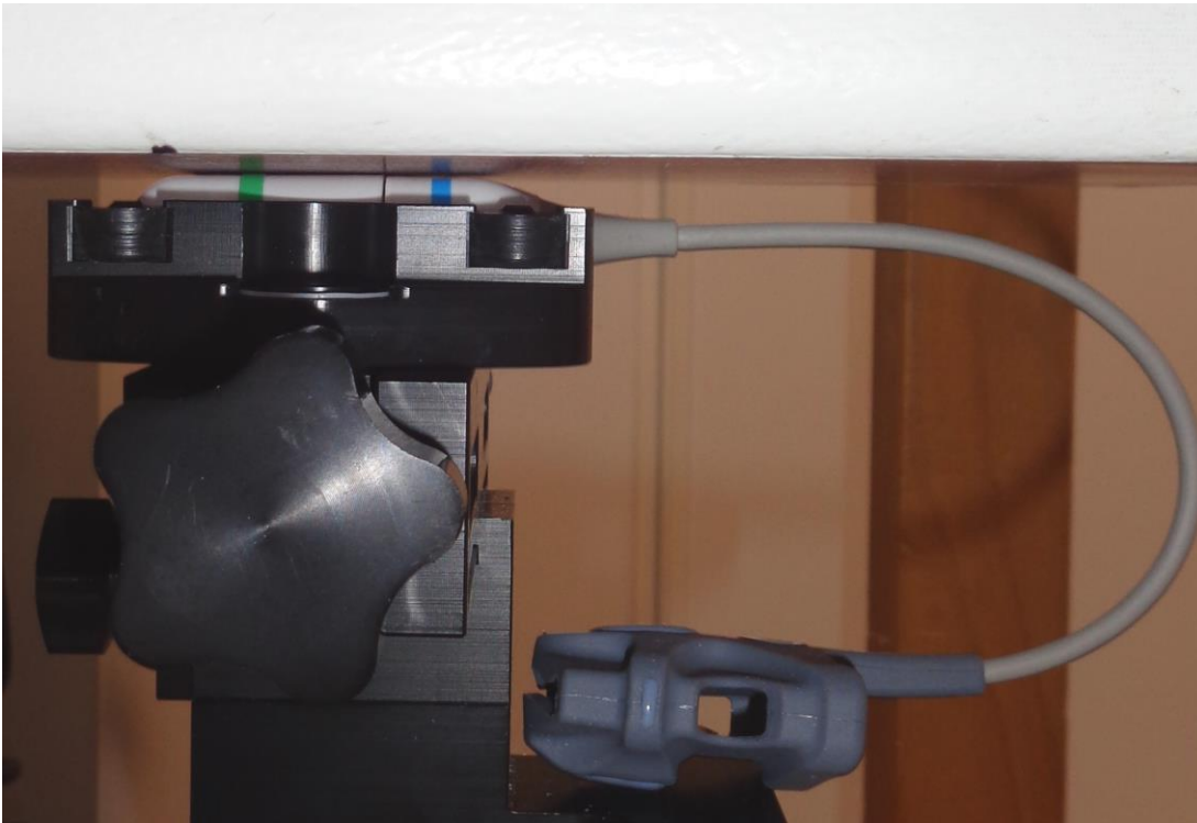
Front side of the Sensor Battery against the phantom, 0mm separation distance
