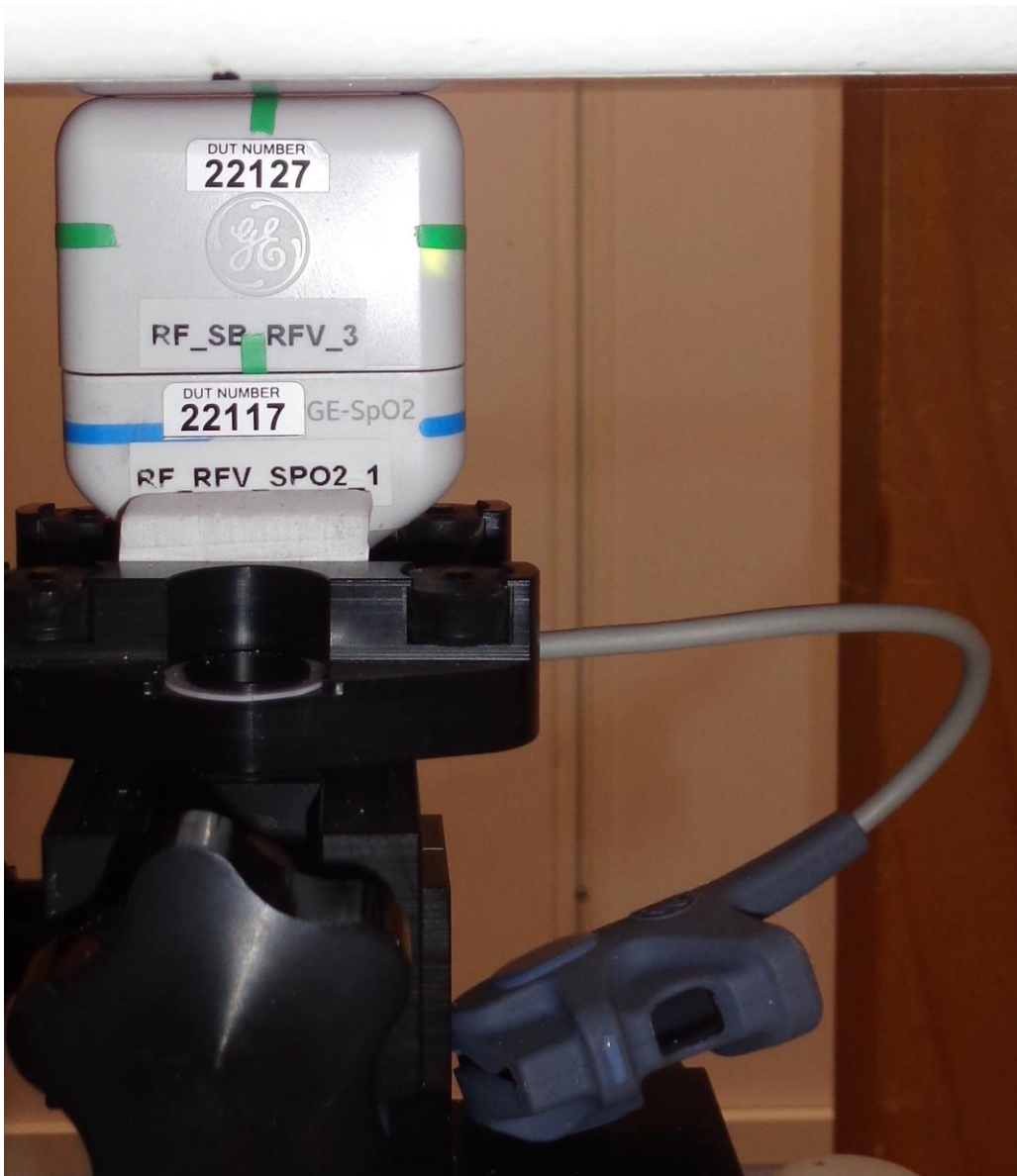
Top side of the Sensor Battery against the phantom, 0mm separation distance
