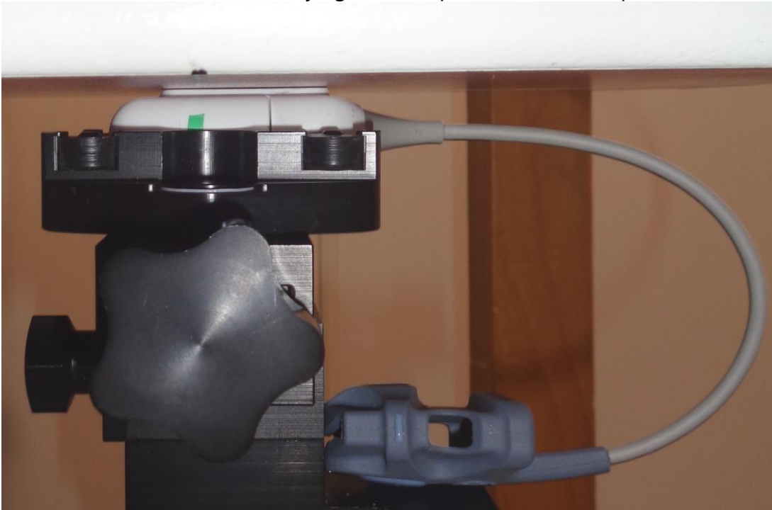
Back side of the Sensor Battery against the phantom, 0mm separation distance
