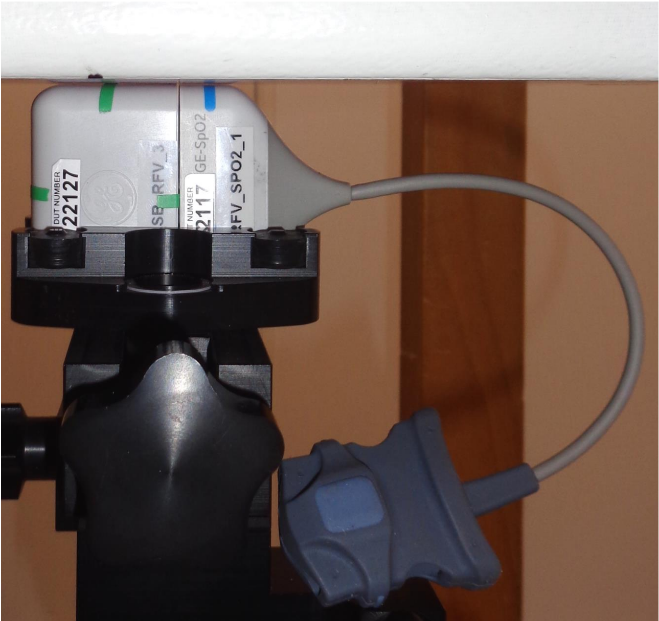
Right side of the Sensor Battery against the phantom, 0mm separation distance
