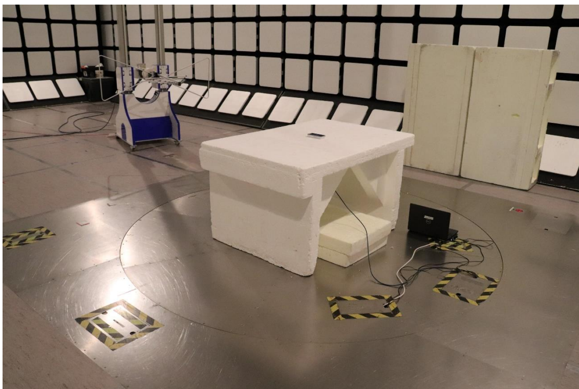
Photograph 2. Test Setup for Radiated Emissions 30 – 1000 MHz
