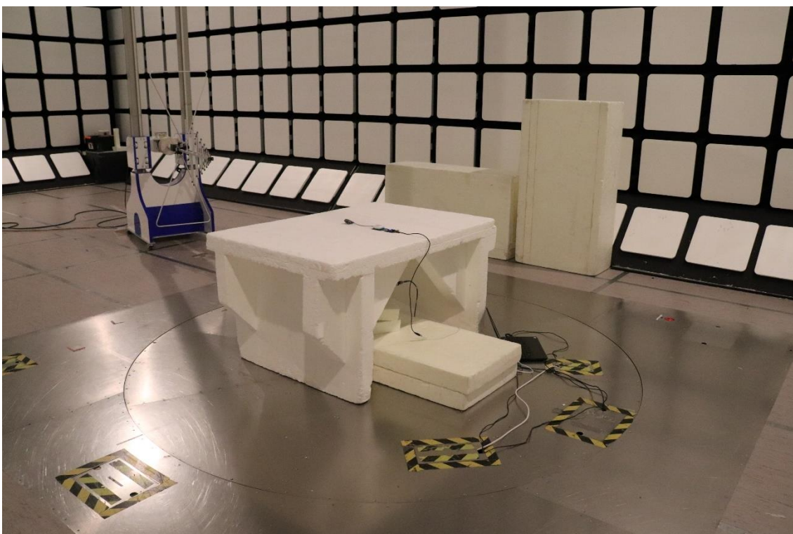
Photograph 2. Test Setup for Radiated Emissions 30 – 1000 MHz
