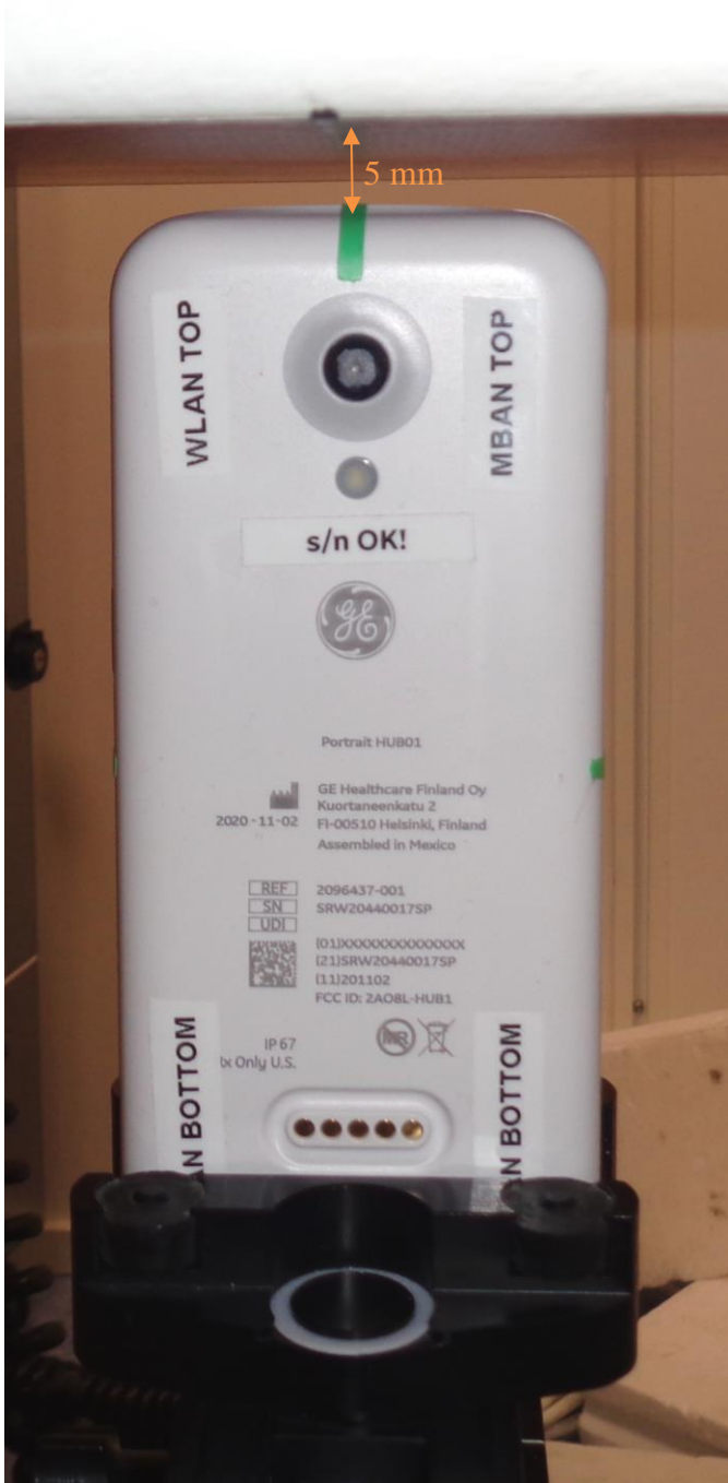
Top side of the HUB against the phantom, 5mm separation distance
