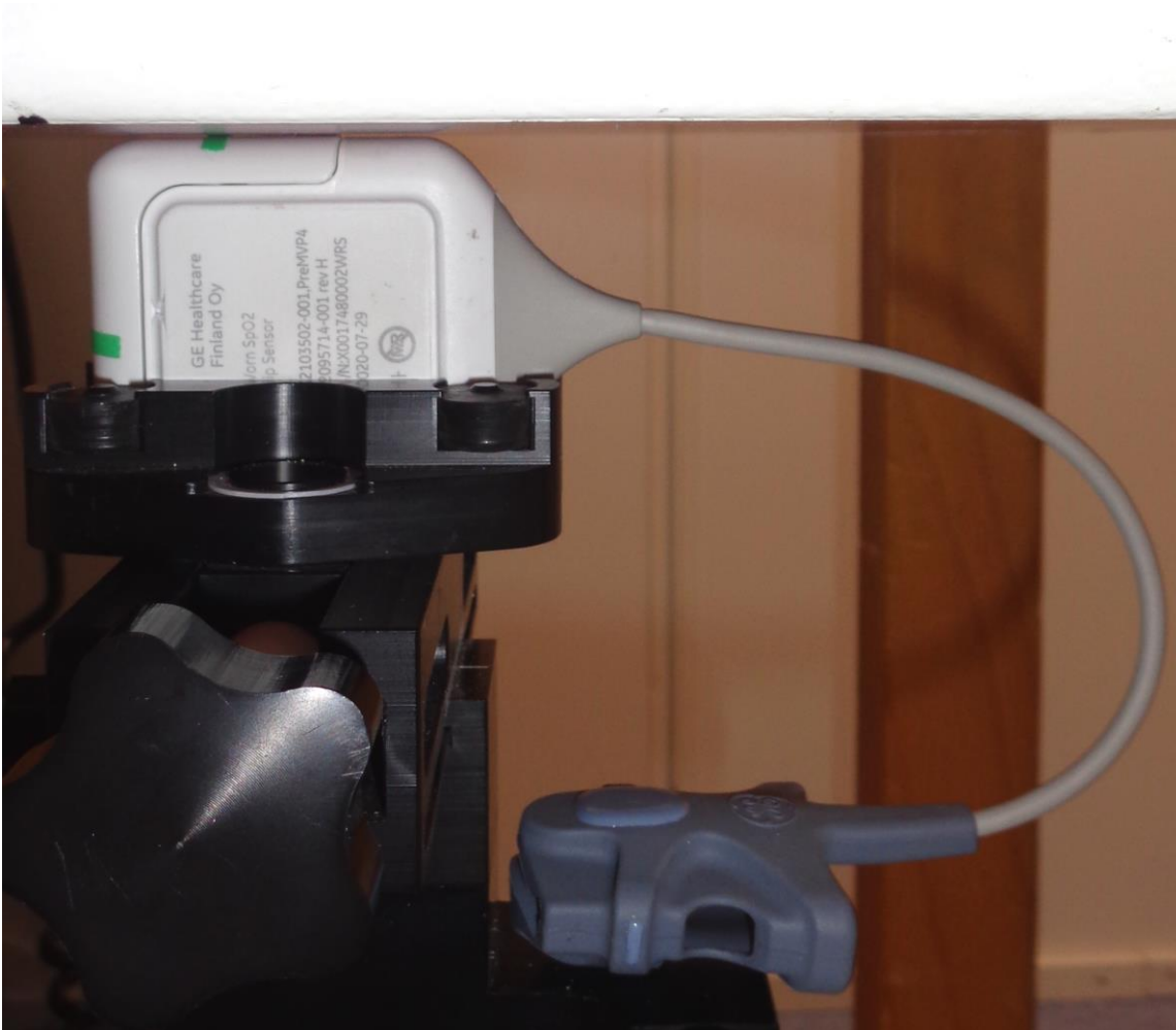
Left side of the Sensor Battery against the phantom, 0mm separation distance
