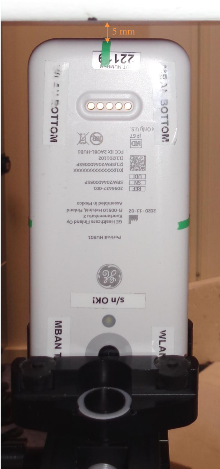
Bottom side of the HUB against the phantom, 5mm separation distance
