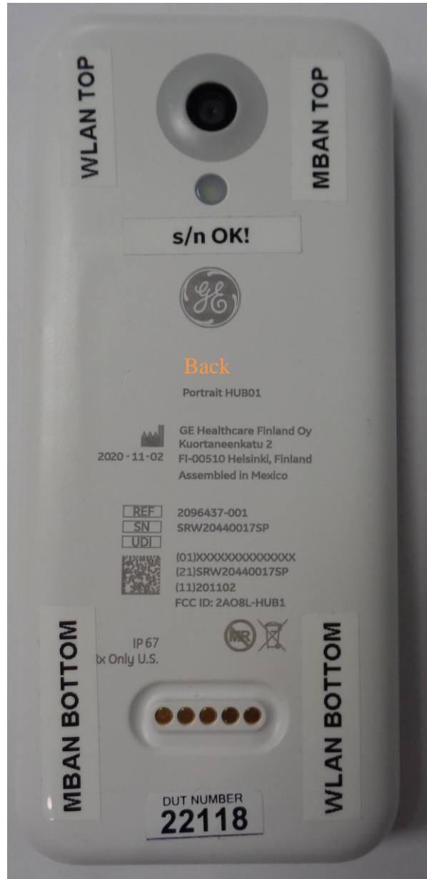
Back side of the HUB and antenna locations
