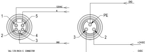
120VAC POWER SUPPLY CONNECTOR FRONT VIEW
