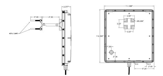
Montage for DV31-DC needs to be done from montage holes on both sides of the box:
