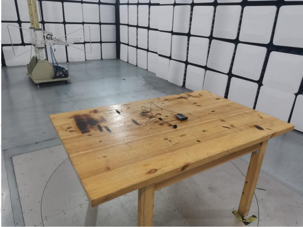
Photo of Radiation Emission Test
