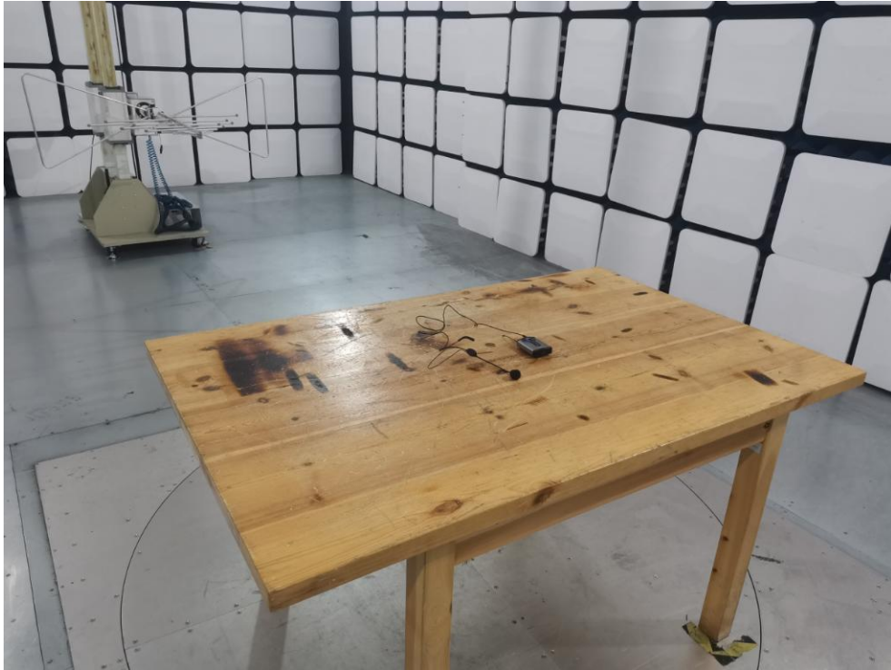
Photo of Radiation Emission Test
