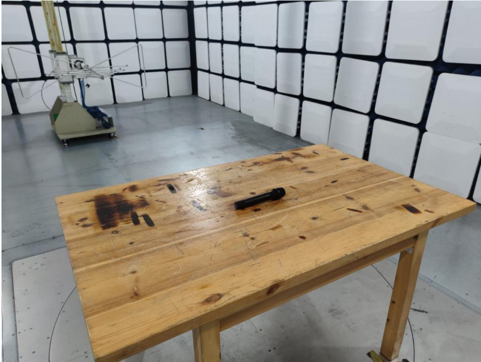
Photo of Radiation Emission Test
