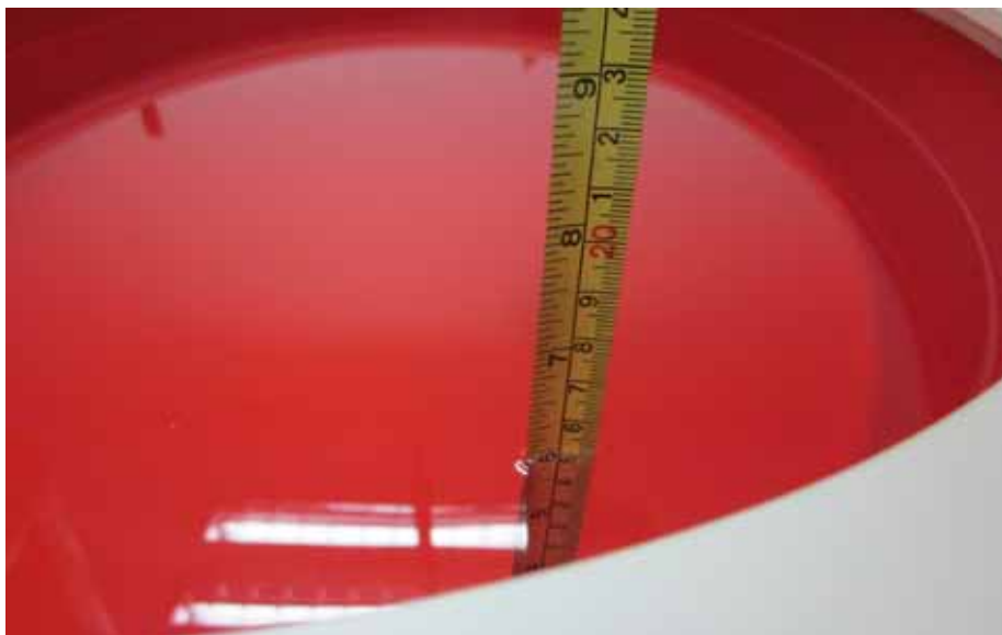
Figure 4.4: Liquid depth in the Flat Phantom
