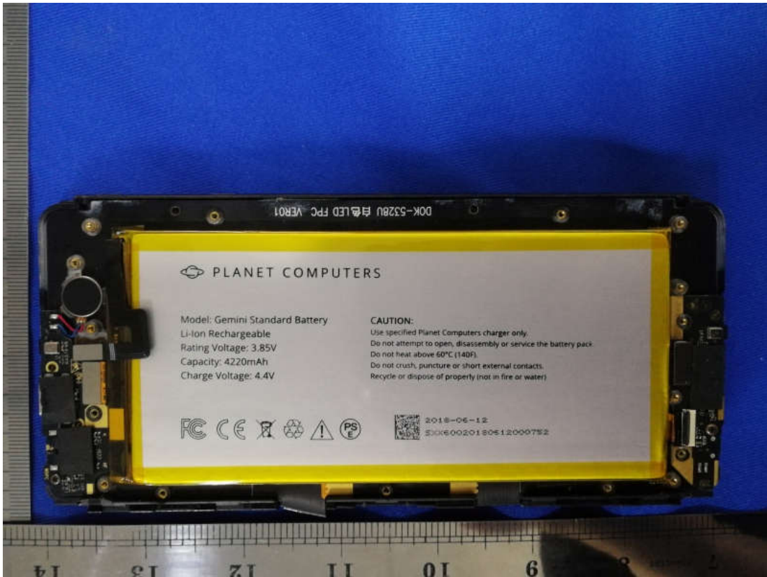
Figure 9 Inside of the EUT
