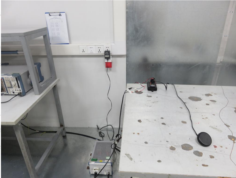
Photo of Power Line Conducted Emission Test
