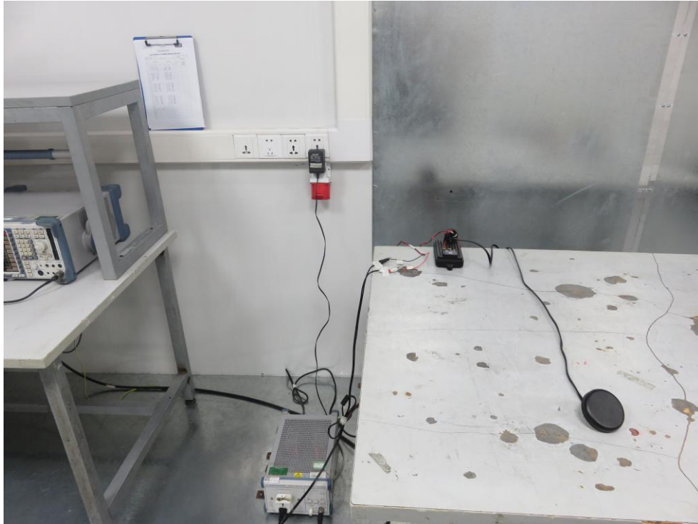
Photo of Conducted Emission Measurement
