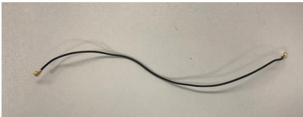
Antenna cable (connected between antenna board and WeMod board)
