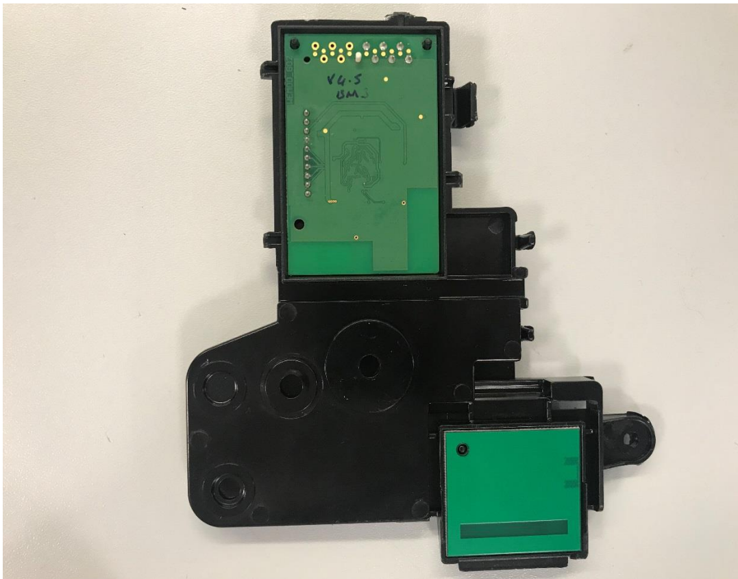
WeMod board and antenna board is located in plastic holder as the following:
