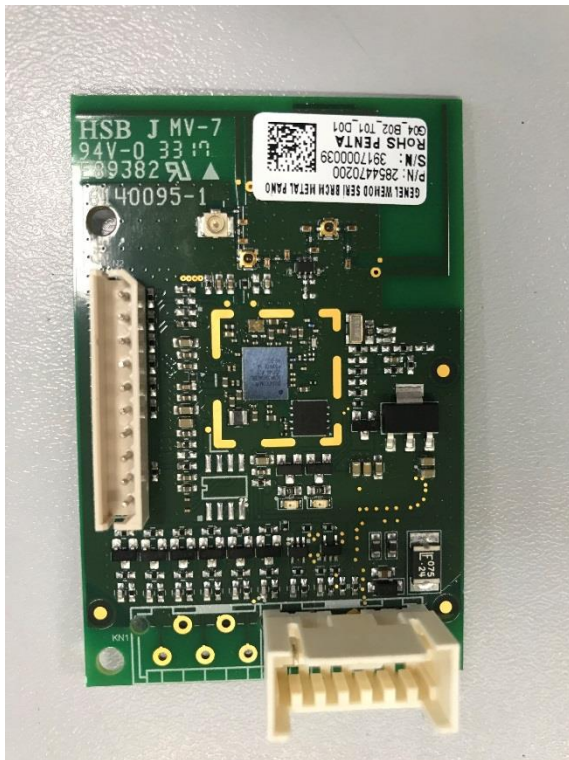
WeMod Board itself (without any holder and cabling)
