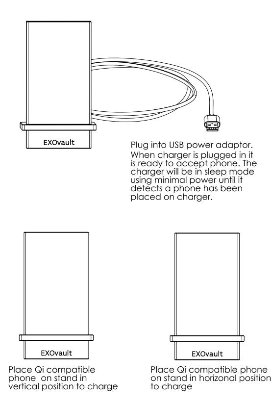
Phone will indicate the charging has begun. Phone will indicate when the phone is fully charged. Charger will automaticly stop charging when phone signals that the phone is full. Charger only works with Qi compatible phones. Non Qi phones will not charge on this stand.
