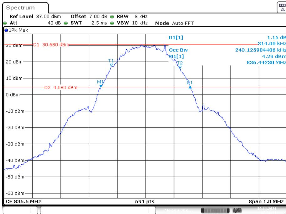
**26 dB Emissions & 99% Occupied Bandwidth for GSM (GMSK) Mode, High channel**
