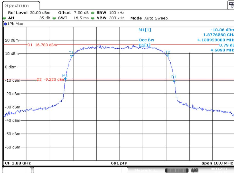
**26 dB Emissions & 99% Occupied Bandwidth for HSUPA (BPSK) Mode, High channel**
