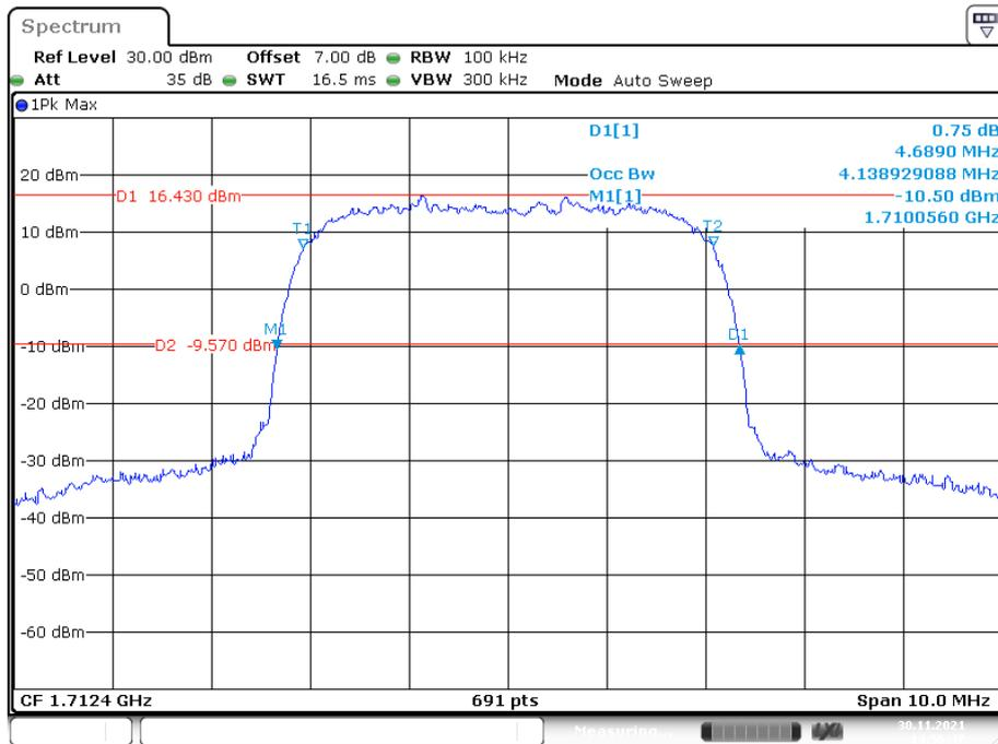
**26 dB Emissions & 99% Occupied Bandwidth for HSUPA (BPSK) Mode, Middle channel**
