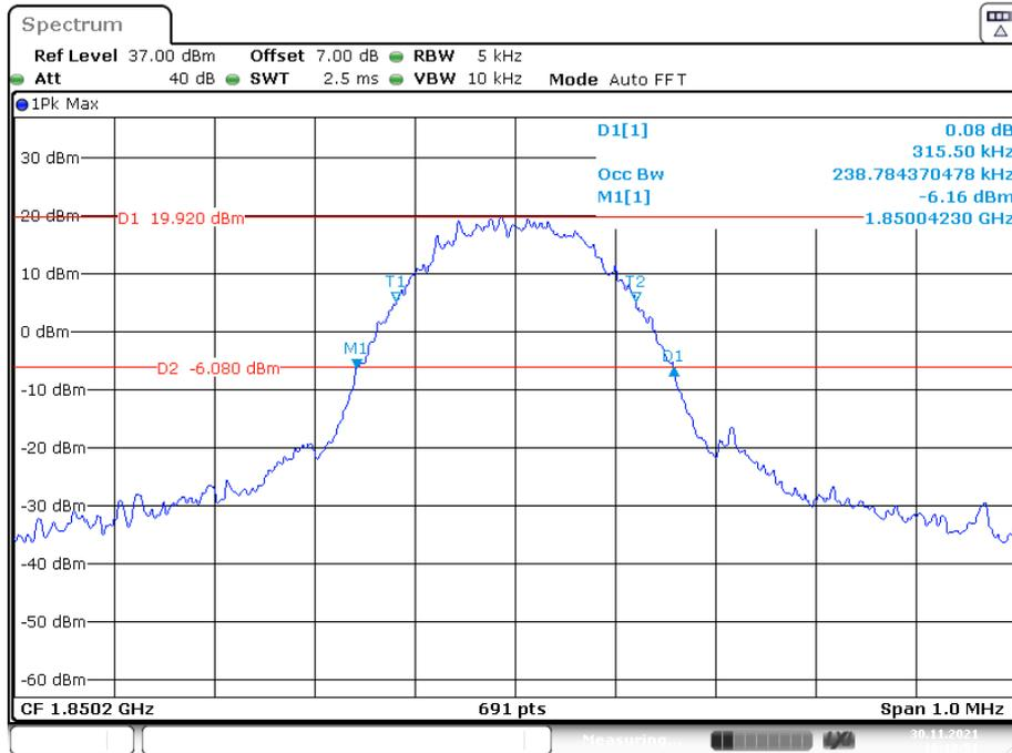
**26 dB Emissions & 99% Occupied Bandwidth for EGPRS (8PSK) Mode, Middle channel**
