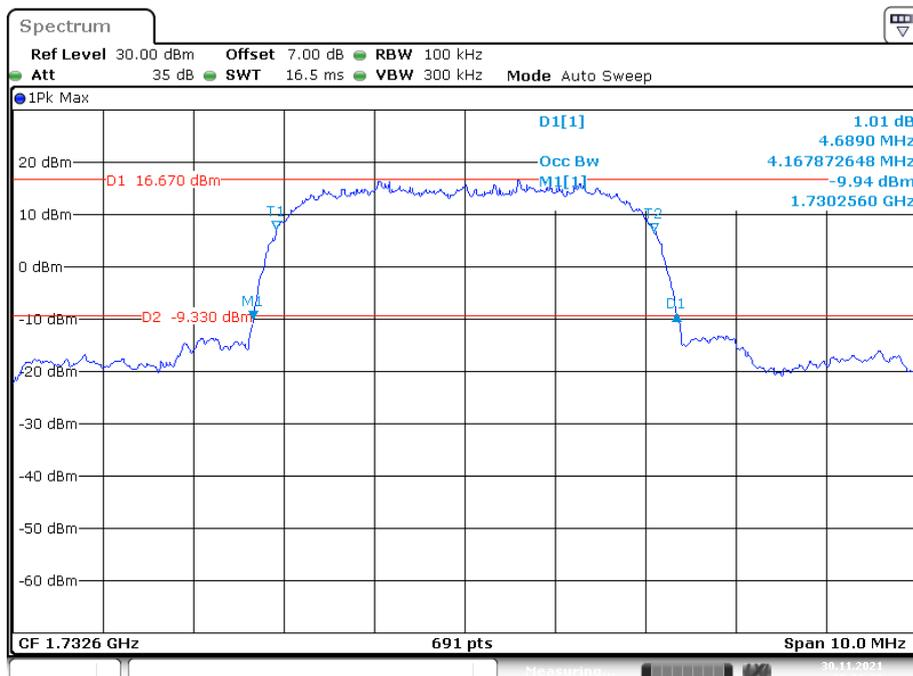
26 dB Emissions & 99% Occupied Bandwidth for HSDPA (16QAM) Mode, High channel
