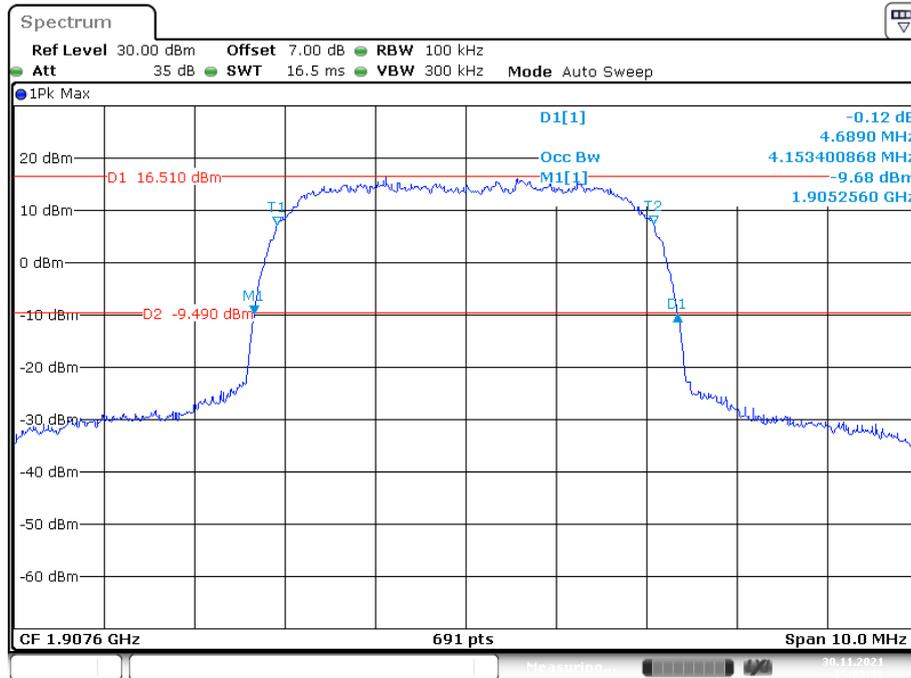
**26 dB Emissions & 99% Occupied Bandwidth for HSDPA (16QAM) Mode, Low channel**
