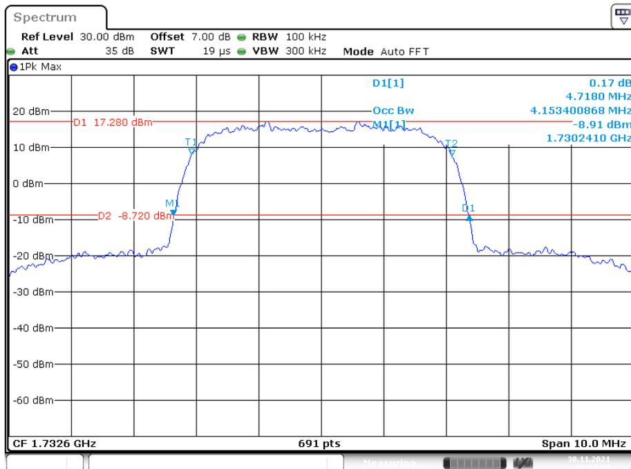
**26 dB Emissions & 99% Occupied Bandwidth for RMC (BPSK) Mode, High channel**
