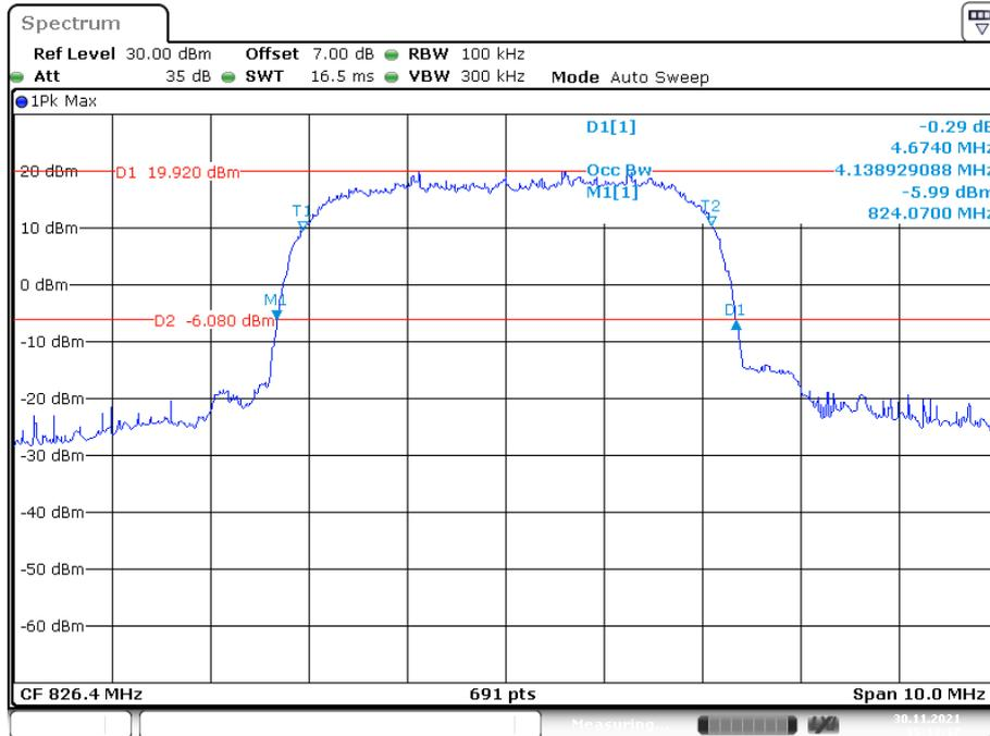
**26 dB Emissions & 99% Occupied Bandwidth for HSDPA (16QAM) Mode, Middle channel**
