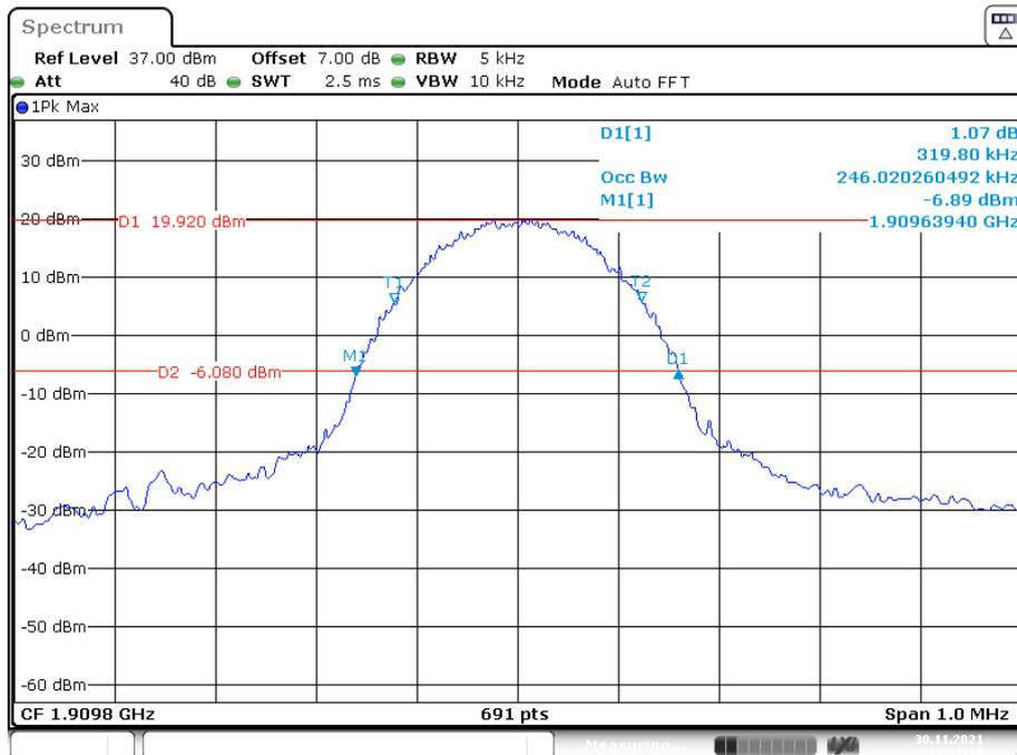
**26 dB Emissions & 99% Occupied Bandwidth for RMC (BPSK) Mode, Low channel**
