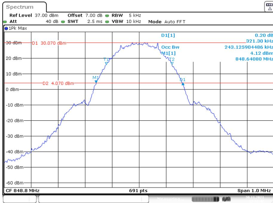
**26 dB Emissions & 99% Occupied Bandwidth for EGPRS (8PSK) Mode, Low channel**
