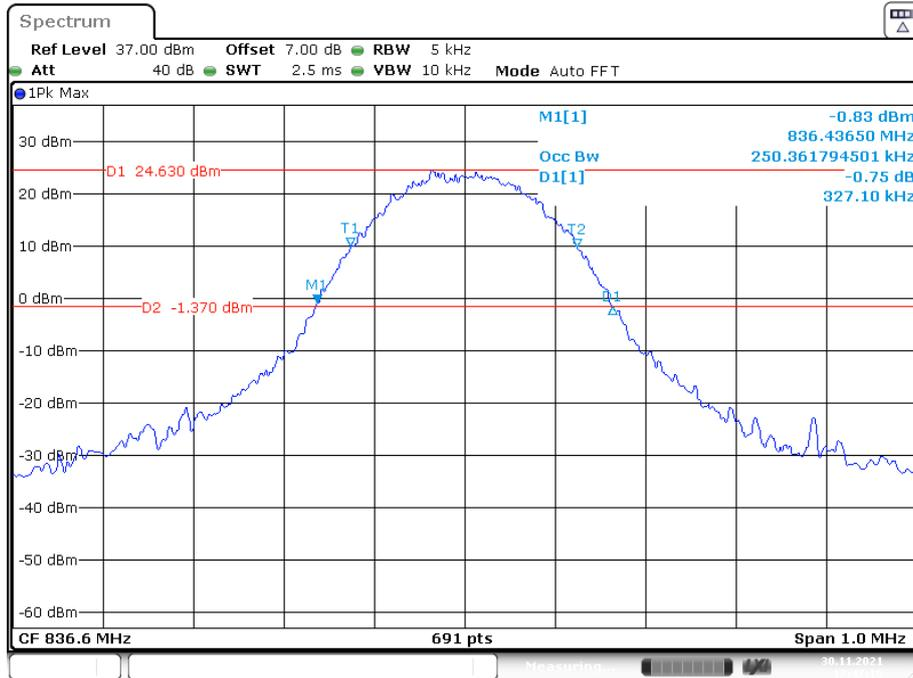
**26 dB Emissions & 99% Occupied Bandwidth for EGPRS (8PSK) Mode, High channel**
