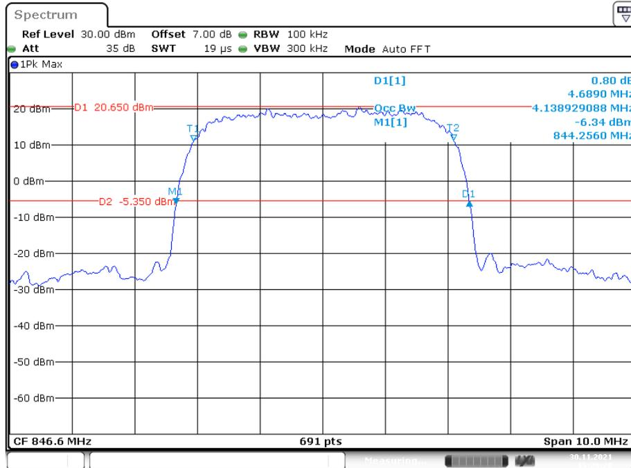
26 dB Emissions & 99% Occupied Bandwidth for HSUPA (BPSK) Mode, Low channel
