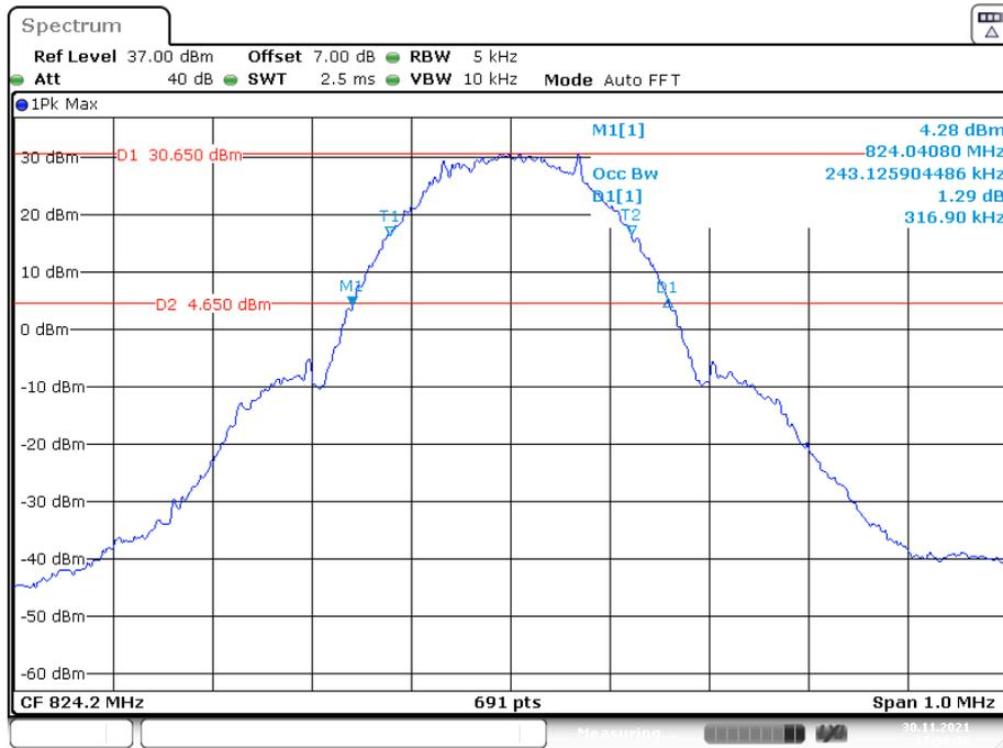
**26 dB Emissions & 99% Occupied Bandwidth for GSM (GMSK) Mode, Middle channel**
