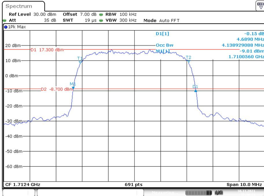
**26 dB Emissions & 99% Occupied Bandwidth for RMC (BPSK) Mode, Middle channel**
