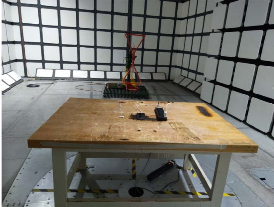
Radiated Emissions View (Below 1 GHz)
