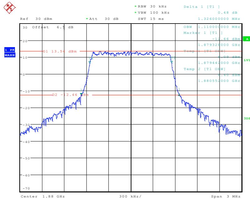
**16-QAM (1.4 MHz) - 26 dB Bandwidth & 99% Occupied Bandwidth, Middle channel**
