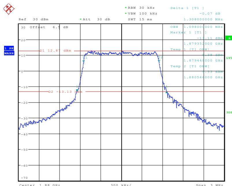
**QPSK (3.0 MHz) - 26 dB Bandwidth & 99% Occupied Bandwidth, Middle channel**
