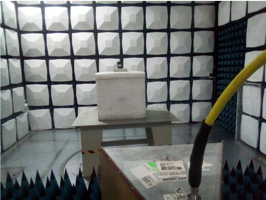
Radiated Emission Above 1GHz View
