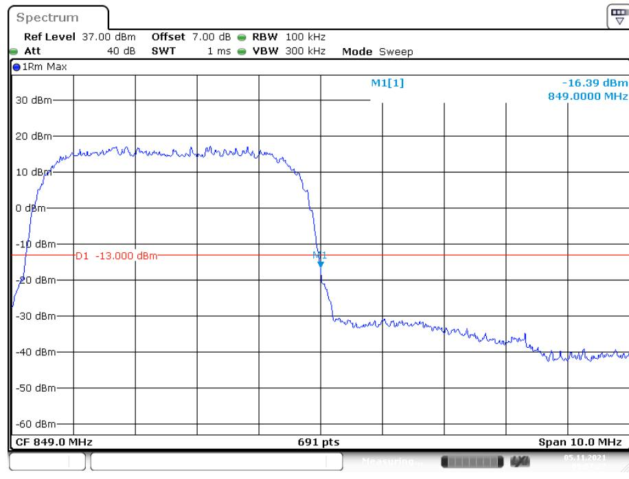
**Cellular Band, Left Band Edge for HSDPA(16QAM) Mode**
