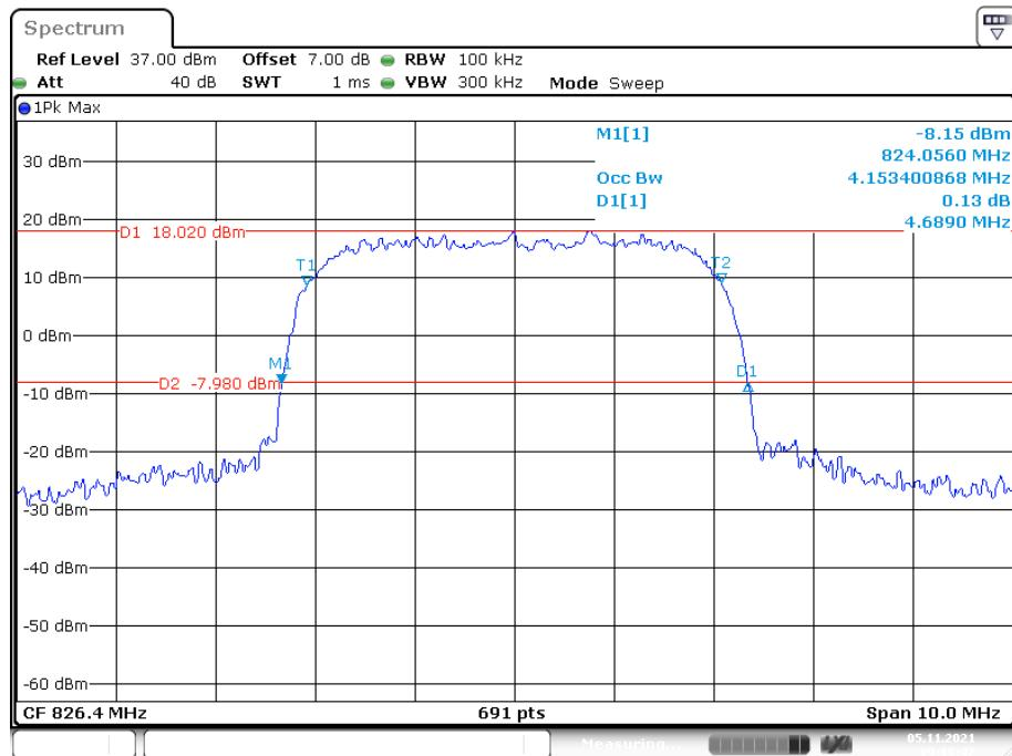
**26 dB Emissions &99% Occupied Bandwidth for HSDPA (16QAM) Mode, Middle channel**
