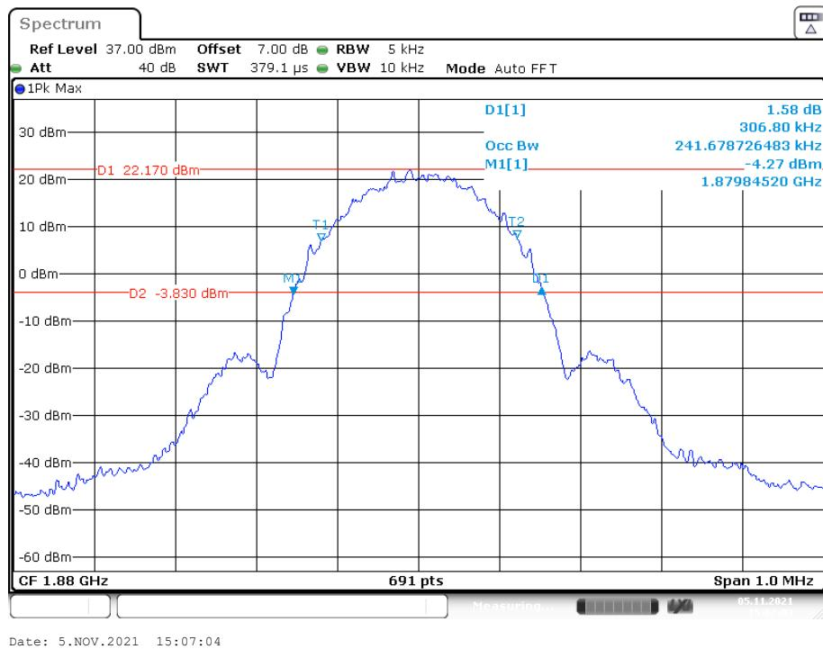
**26 dB Emissions &99% Occupied Bandwidth for EGPRS (8PSK) Mode, High channel**
