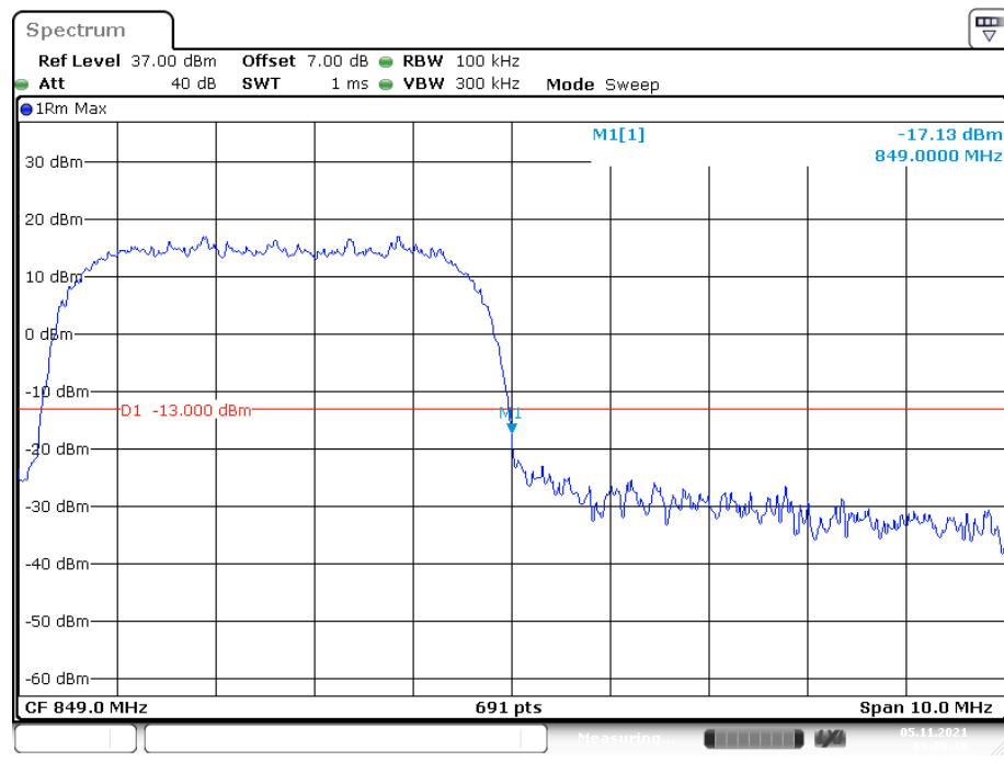
**Cellular Band, Left Band Edge for HSUPA (BPSK) Mode**
