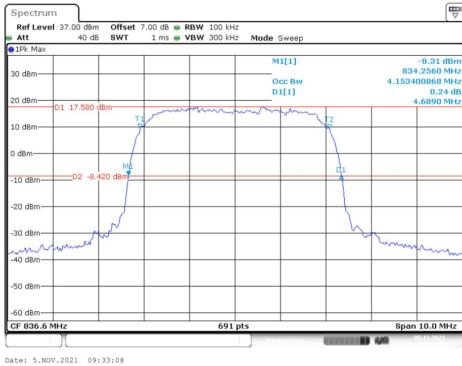
**26 dB Emissions &99% Occupied Bandwidth for HSUPA (BPSK) Mode, High channel**
