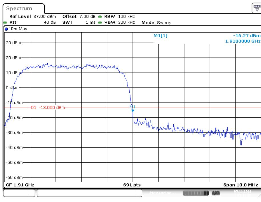
**PCS Band, Left Band Edge for HSUPA (BPSK) Mode**
