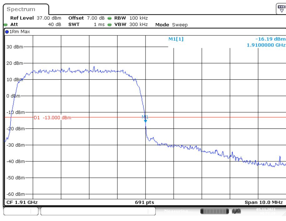
**PCS Band, Left Band Edge forHSDPA(16QAM) Mode**
