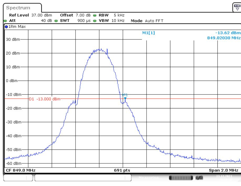
**Cellular Band, Left Band Edge for EGPRS (8PSK) Mode**
