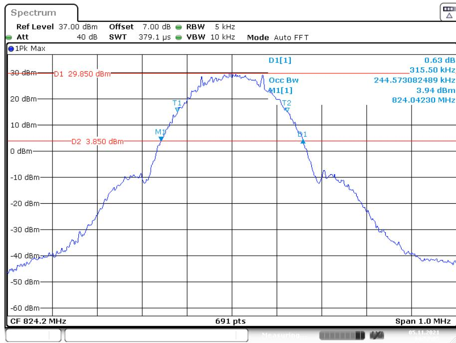
**26 dB Emissions &99% Occupied Bandwidth for GSM (GMSK) Mode, Middle channel**
