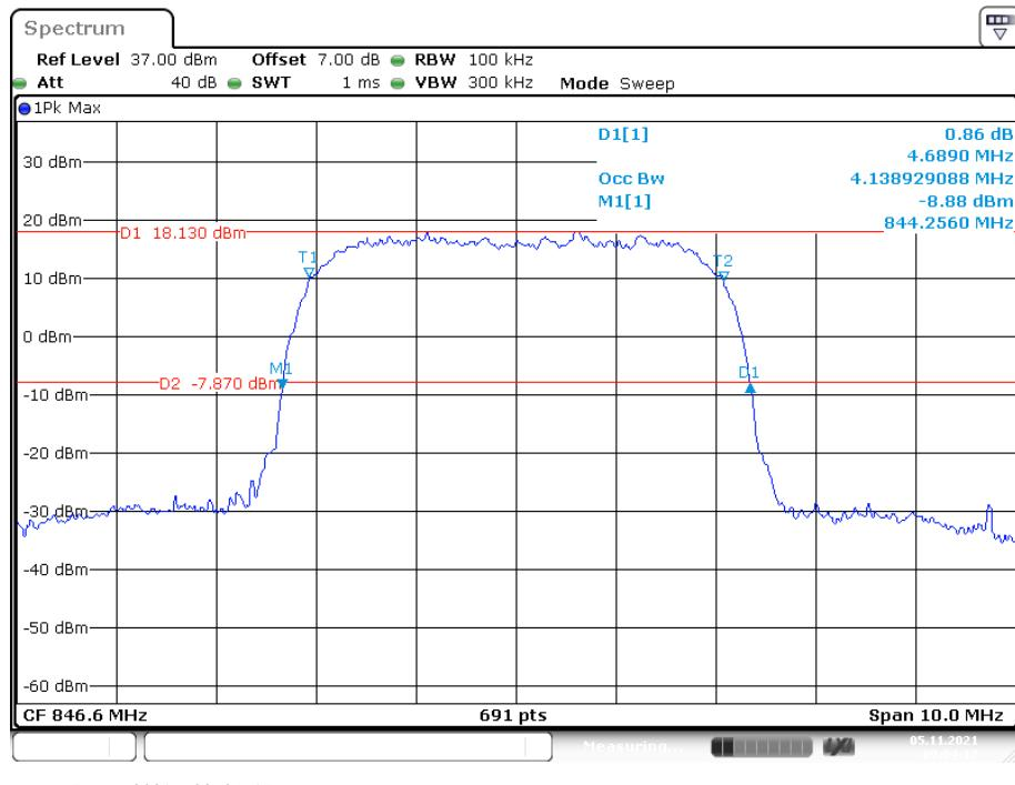
**26 dB Emissions &99% Occupied Bandwidth for HSUPA (BPSK) Mode, Low channel**
