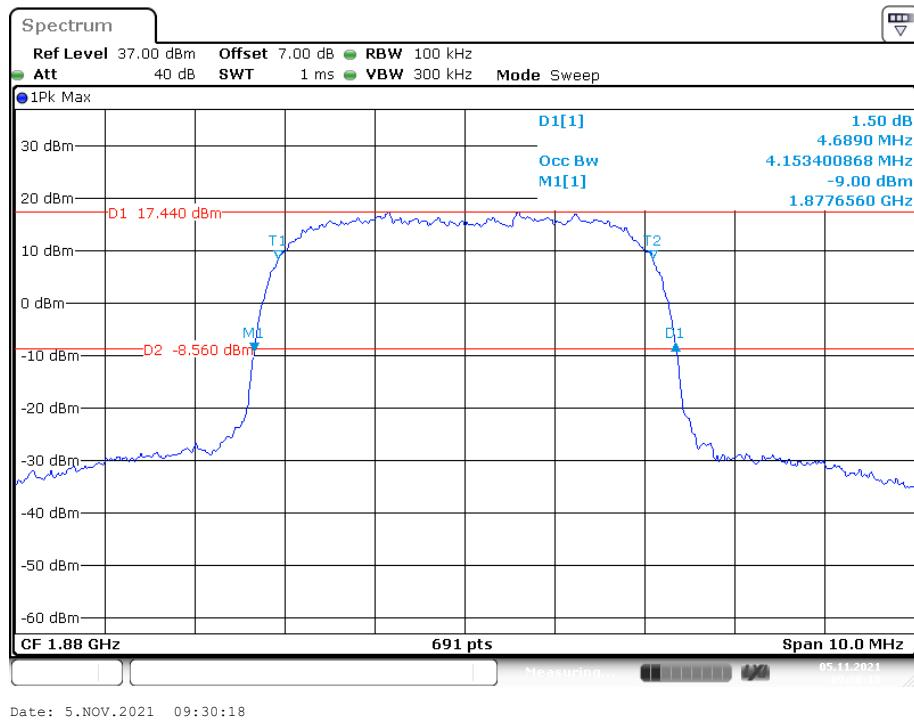
**26 dB Emissions &99% Occupied Bandwidth for HSUPA (BPSK) Mode, High channel**
