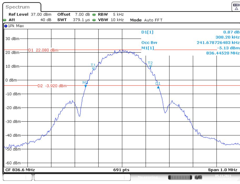
**26 dB Emissions &99% Occupied Bandwidth for EGPRS (8PSK) Mode, High channel**
