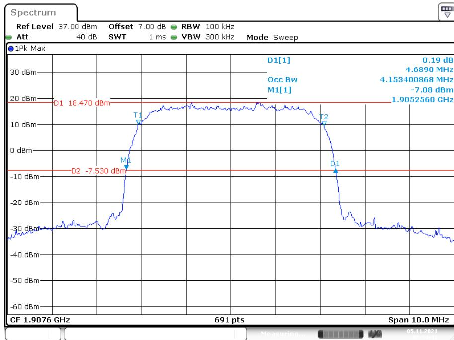
**26 dB Emissions &99% Occupied Bandwidth for HSUPA (BPSK) Mode, Low channel**
