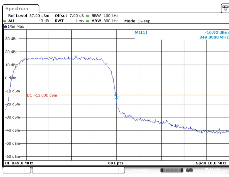
**PCS Band, Left Band Edge for GSM (GMSK) Mode**
