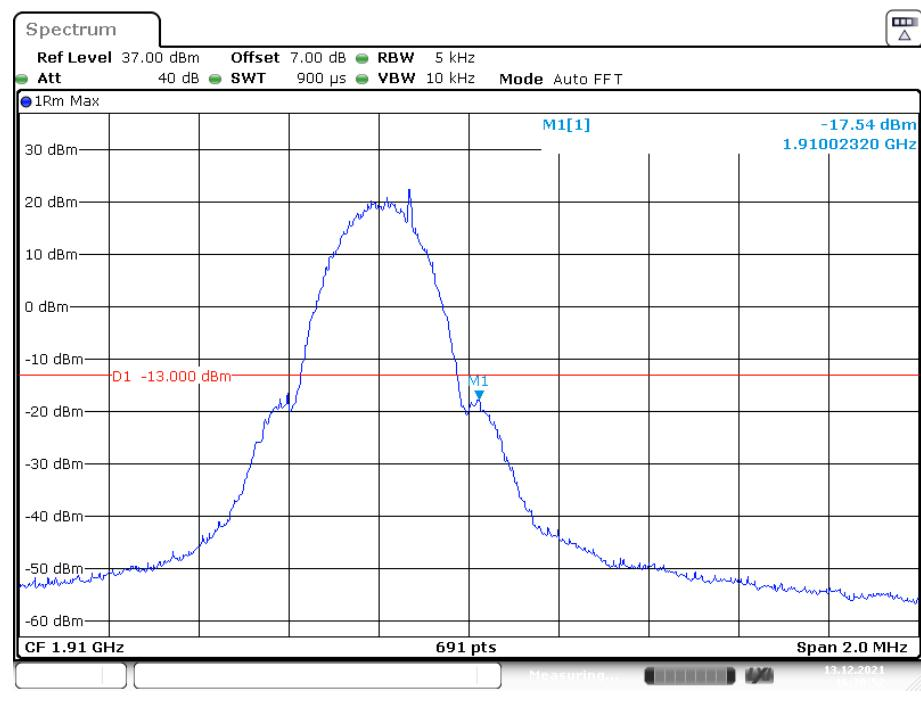
**PCS Band, Left Band Edge for EGPRS (8PSK) Mode**
