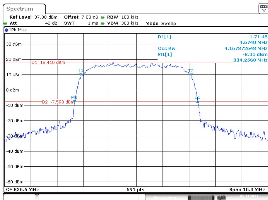
**26 dB Emissions &99% Occupied Bandwidth for HSDPA (16QAM) Mode, High channel**
