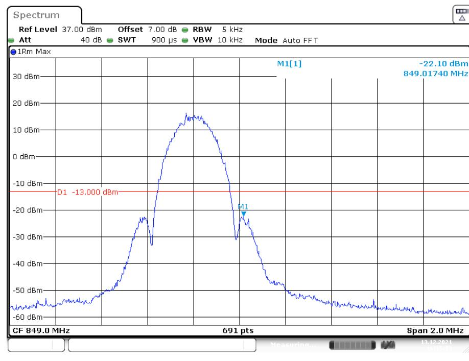
**Cellular Band, Left Band Edge for RMC (BPSK) Mode**
