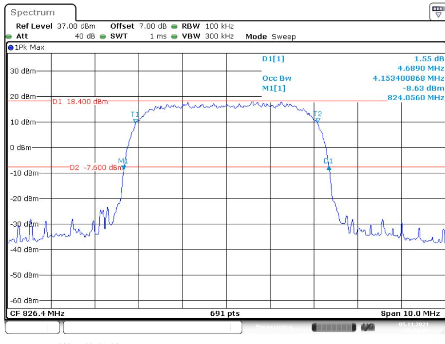
**26 dB Emissions &99% Occupied Bandwidth for RMC (BPSK) Mode, Middle channel**
