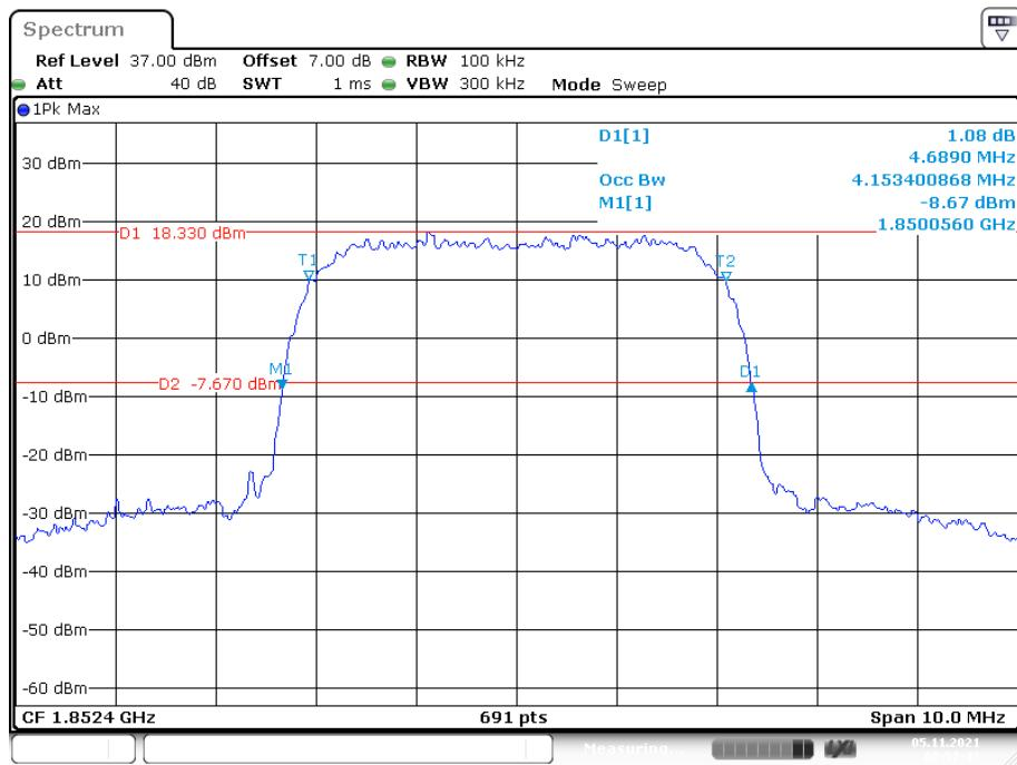
**26 dB Emissions &99% Occupied Bandwidth for RMC (BPSK) Mode, Middle channel**
