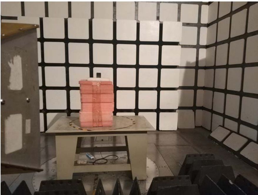
Radiated Emissions View (Above 1 GHz)
