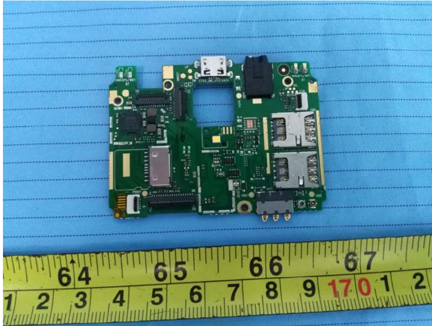
EUT – Main Board Top Shielding off View
