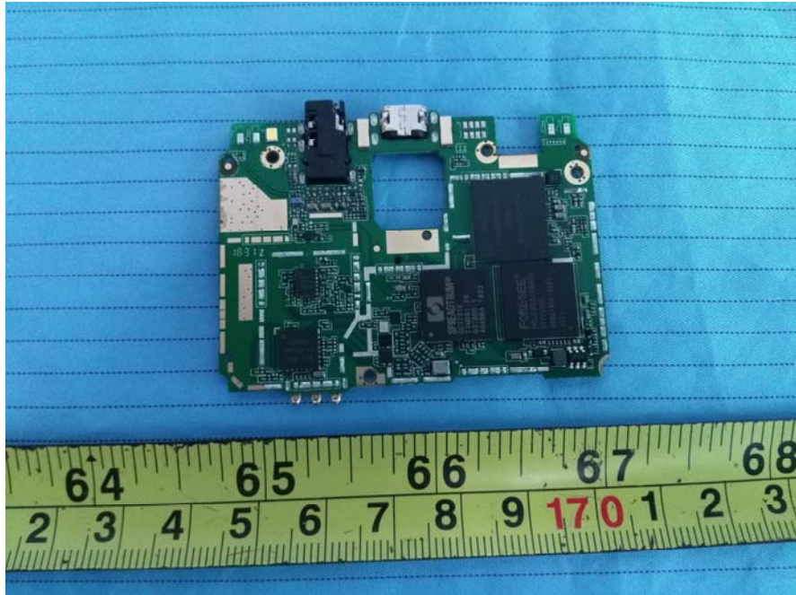
EUT – Main Board Bottom Shielding off View
