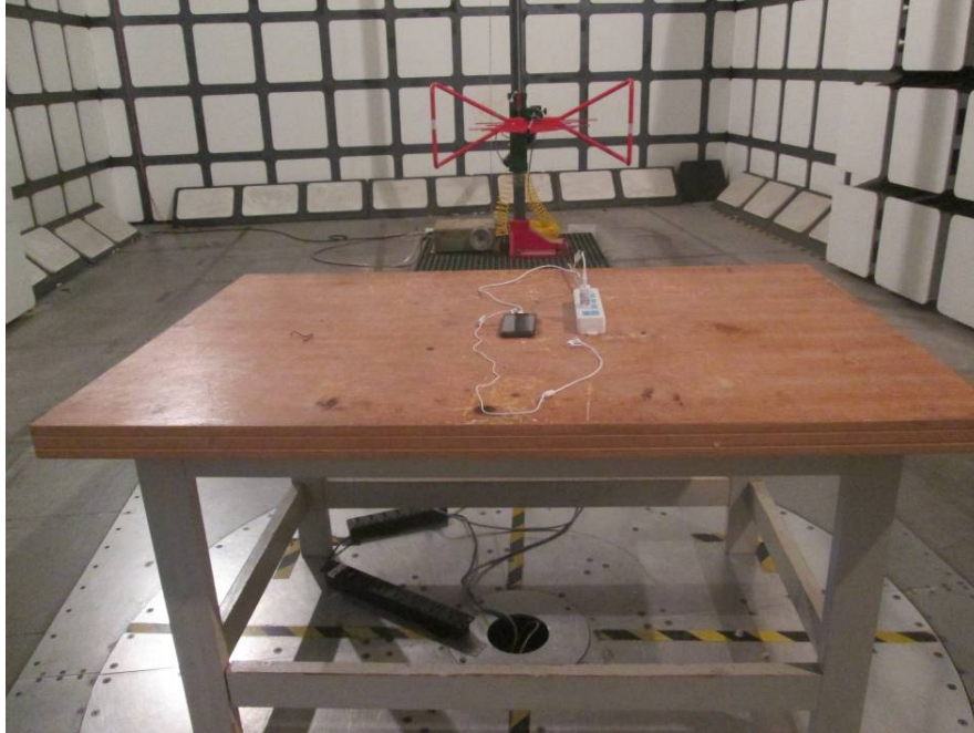
Radiated Emissions View (Below 1 GHz)
