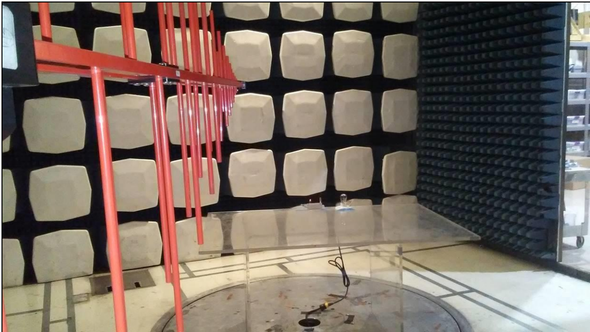
Photograph 7. Radiated Emissions, Setup Below 1GHz - 3w Dimmer
