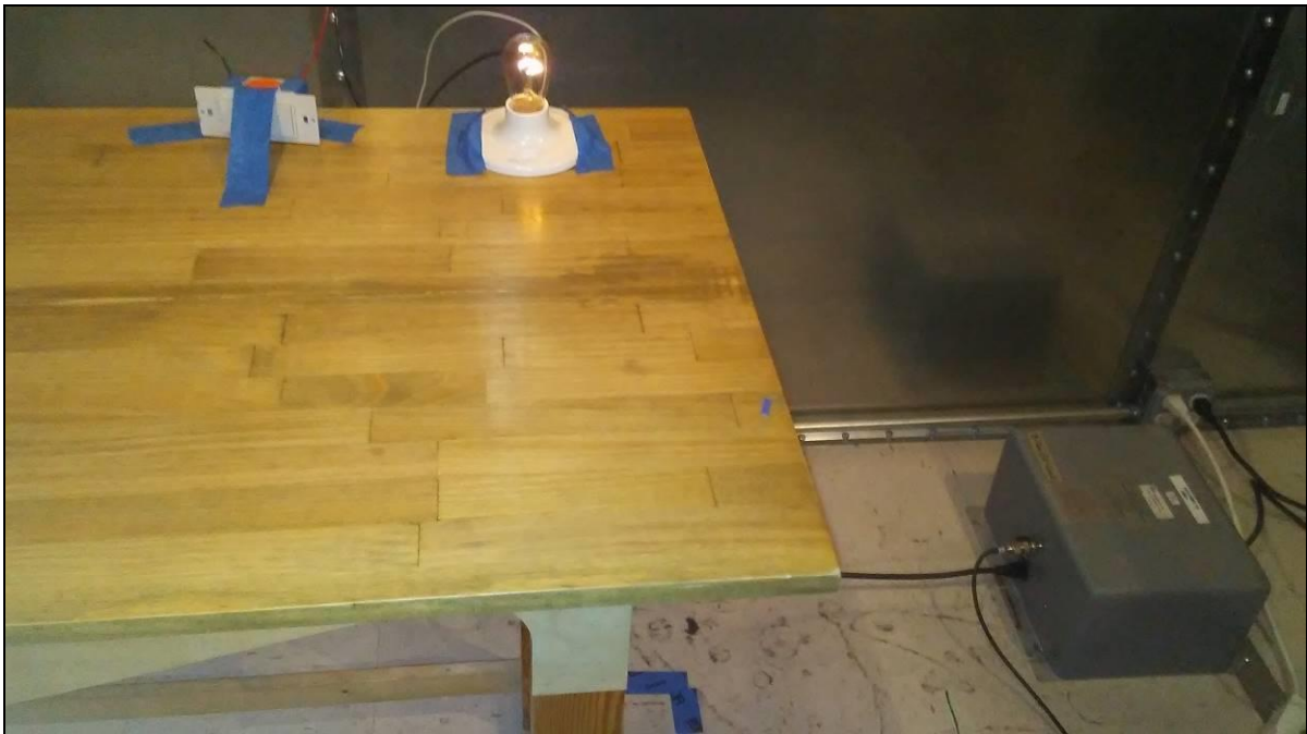
Photograph 2. Conducted Emissions, 15.207(a), 3 wire dimmer, Test Setup
