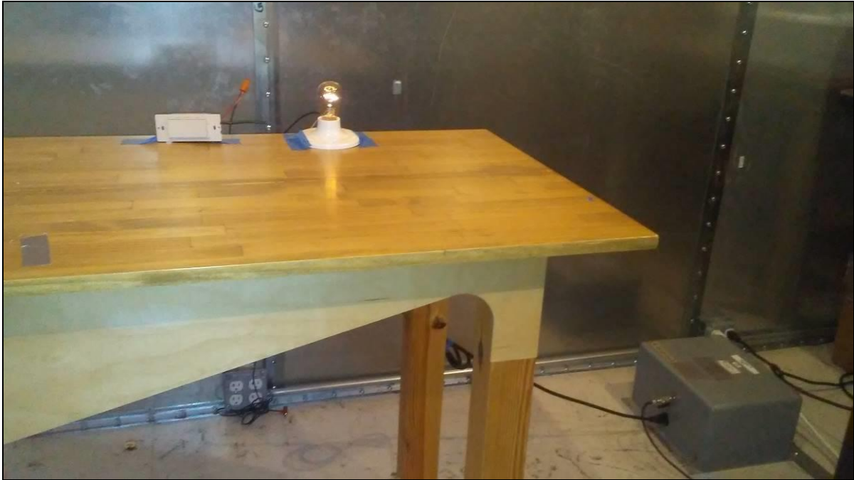
Photograph 1. Conducted Emissions, 15.207(a), 2 wire dimmer, Test Setup
