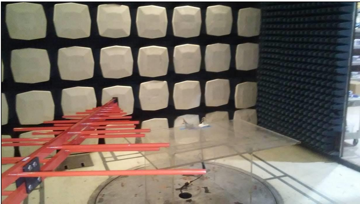
Photograph 9. Radiated Emissions, Setup Below 1GHz - Switch
