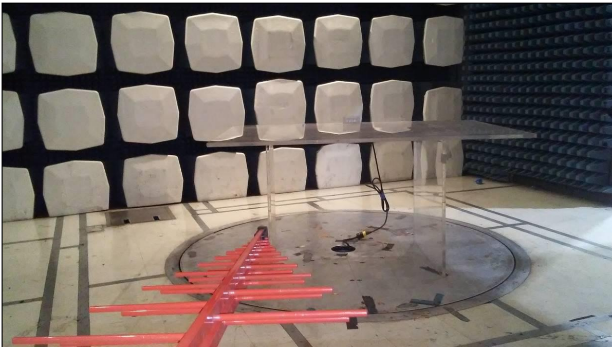
Photograph 11. Radiated Emissions, Setup Below 1GHz - Keypad
