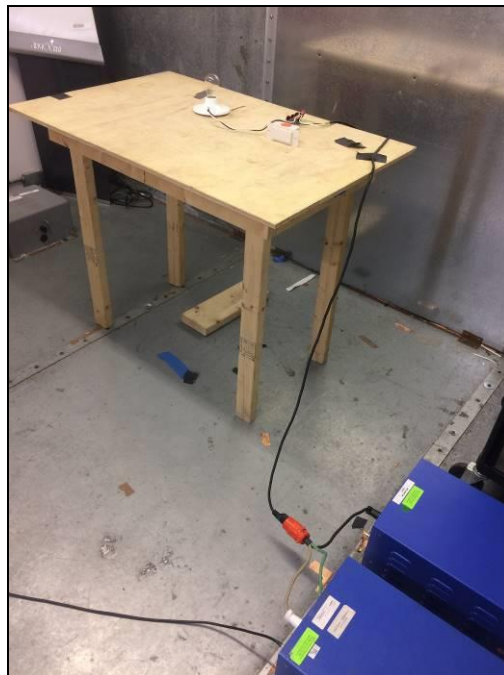
Photograph 4. Conducted Emissions, 15.207(a), Standard Switch, Test Setup
