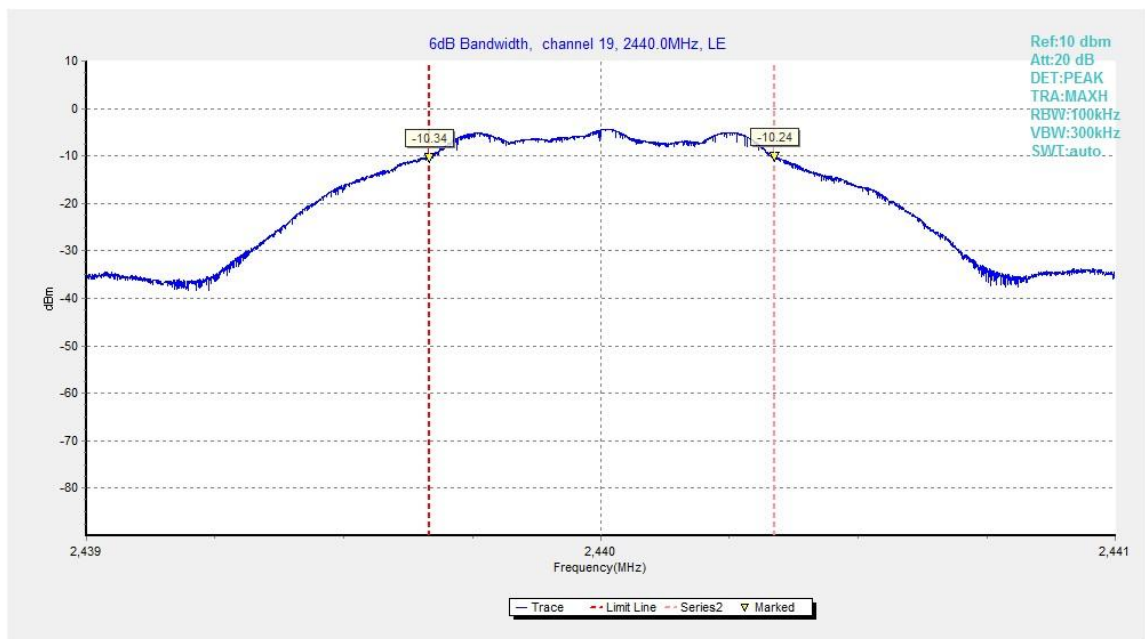
Fig.21. 6dB Bandwidth: GFSK, 2440 MHz
