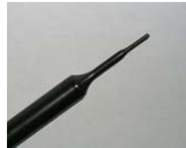
Picture C.2 Near-field Probe
