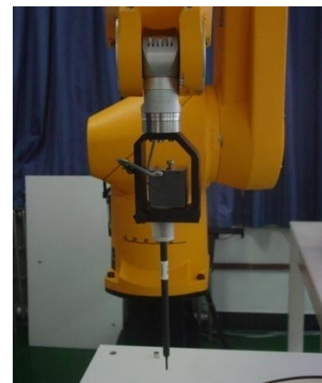
Picture C.3 E-field Probe
