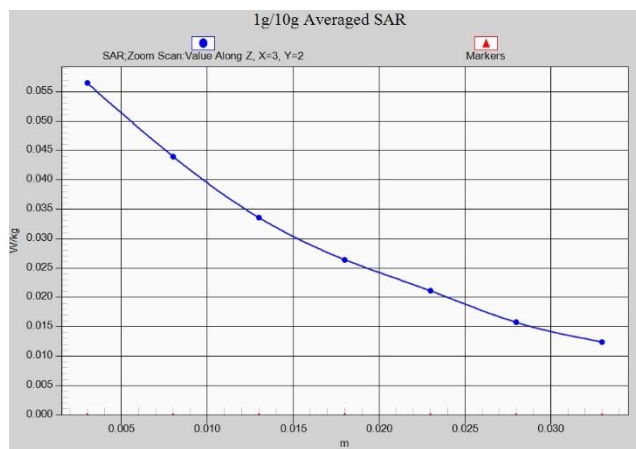
Fig.A.1- 11 Z-Scan at power reference point (LTE Band12)
