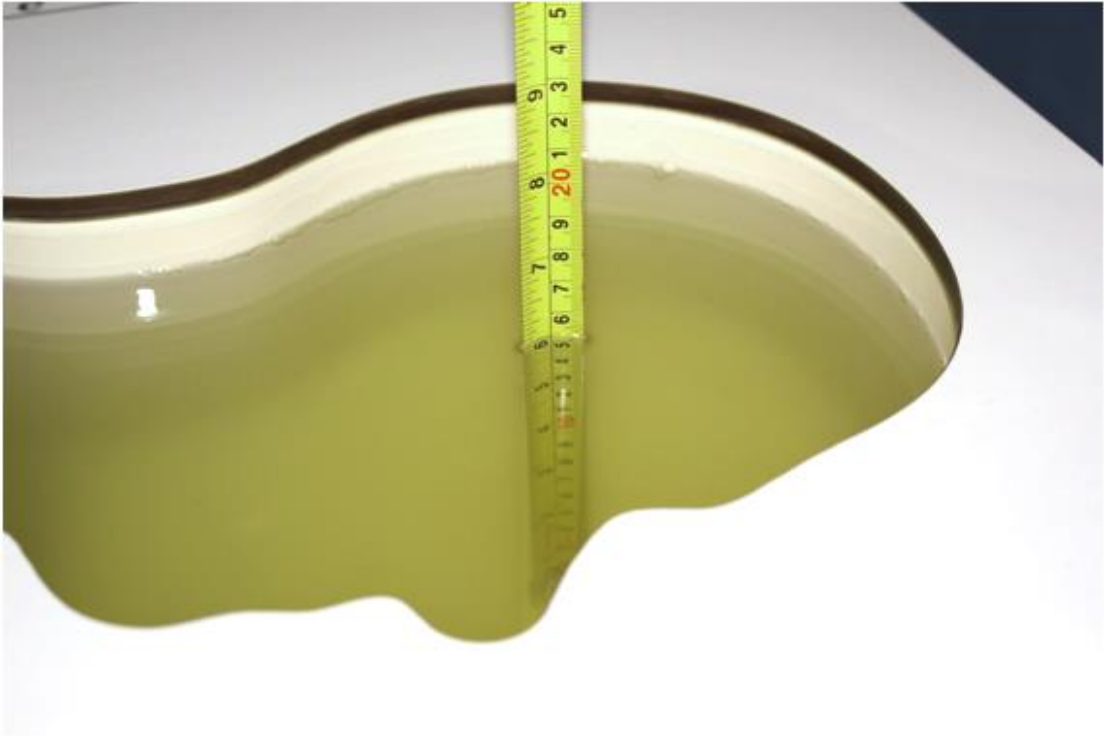
Picture 7-11 Liquid depth in the Head Phantom (2300 MHz Head)
