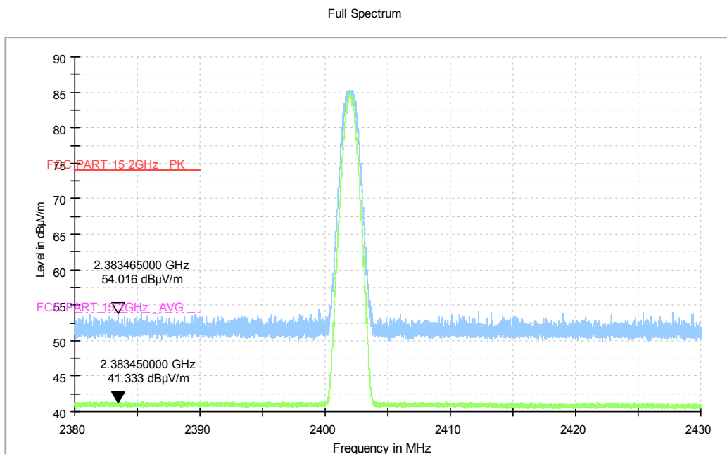
Fig.60. Radiated emission (Power): \pi/4 DQPSK, low channel
