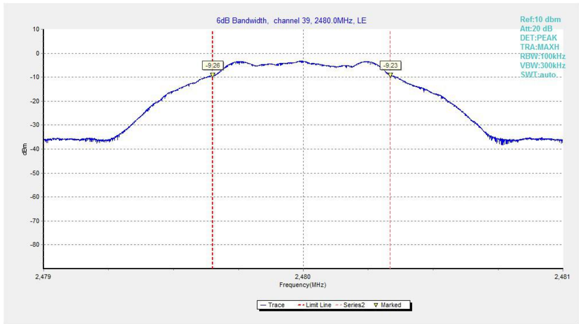
Fig.22. 6dB Bandwidth: GFSK, 2480 MHz
