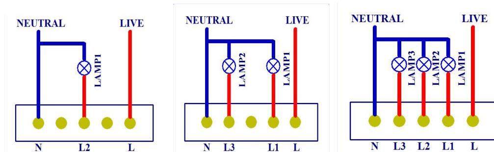
A switch wiring diagram
