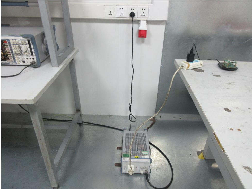
Photo of Conducted Emission Measurement
