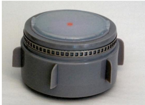
Picture 5 Sensor with red LED indicating successful sensor registration
