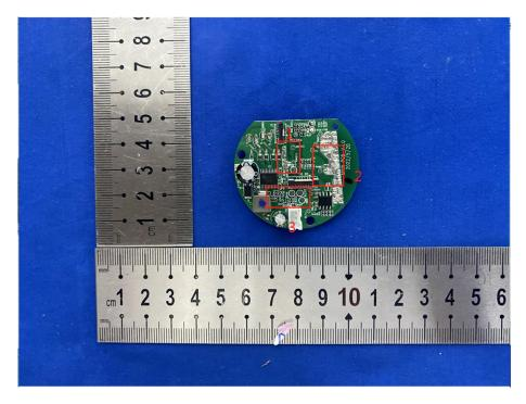
Note: Location 1 and location 2 have changed wiring, and location 3 has added components
