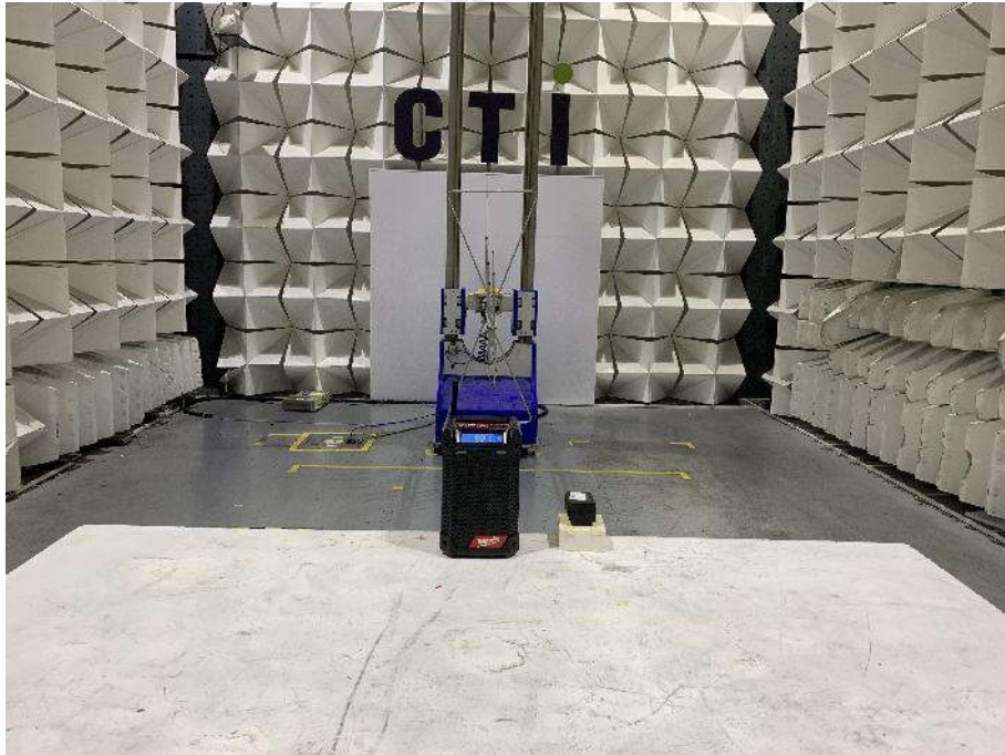
Radiated spurious emission Test Setup-1(Below 1GHz)
