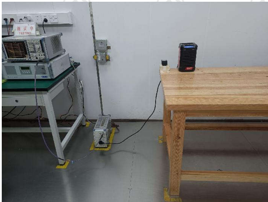
Conducted Emissions Test Setup
