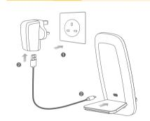
$\ensuremath{\textcircled{1}}$  Connect the power adapter to socket. ② Connect adapter to the USB 2.0 interface, the other Micro USB to transmitter, LED light become green and enter to standby mode.
