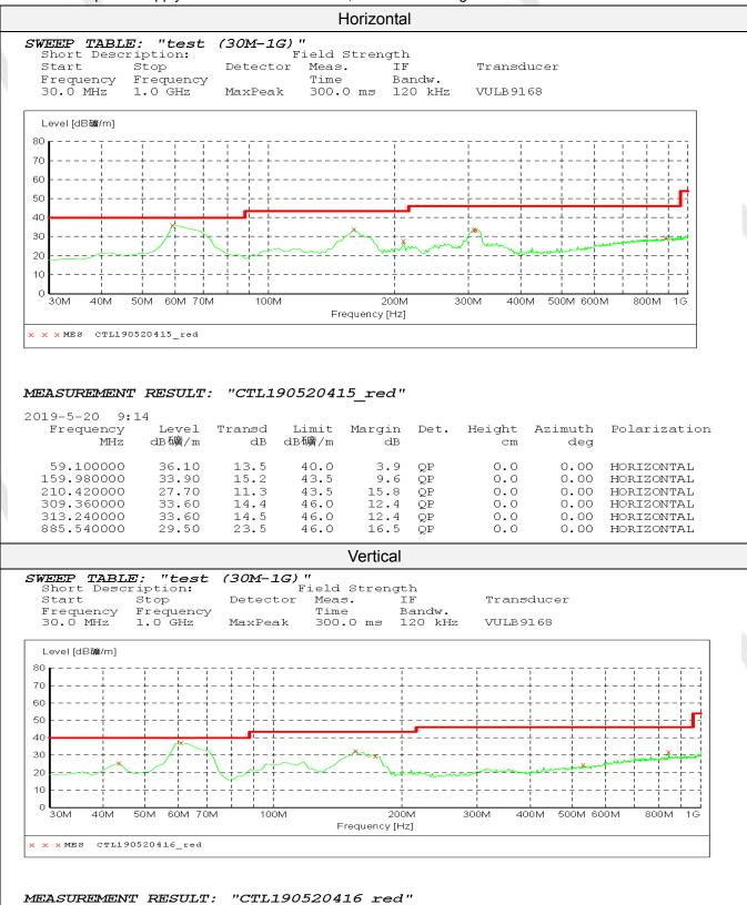
2019-5-20 9:16 Frequency Height Azimuth Level Transd Limit Margin Det. Polarization MHz dB礦/m dB礦/m dB deg dB сm 43.580000 25.50 14.5 13.2 40.0 14.5 0.0 0.00 VERTICAL OP 34.20 40.0 5.8 QΡ 61.040000 0.0 0.00 VERTICAL 15.2 13.7 156.100000 32.60 43.5 10.9 QP 0.0 0.00 VERTICAL 173.560000 532.460000 842.860000 29.50 43.5 14.0 QP 0.0 0.00 VERTICAL 24.60 31.80 QΡ QΡ 46.0 46.0 21.4 14.2 0.00 VEBTICAL 18.8 0.0 23.0 0.0 VERTICAL
