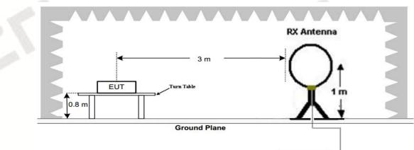
2. Radiated Emission Test Set-Up, Frequency below 1000MHz
