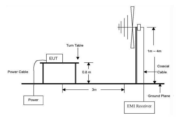
The diagram below shows the test setup that is utilized to make the measurements for emission from 1  $\mathbb{G}_2$  to 40  $\mathbb{G}_2$  emissions.
