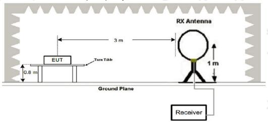
2. Radiated Emission Test-Up Frequency 30MHz~1GHz
