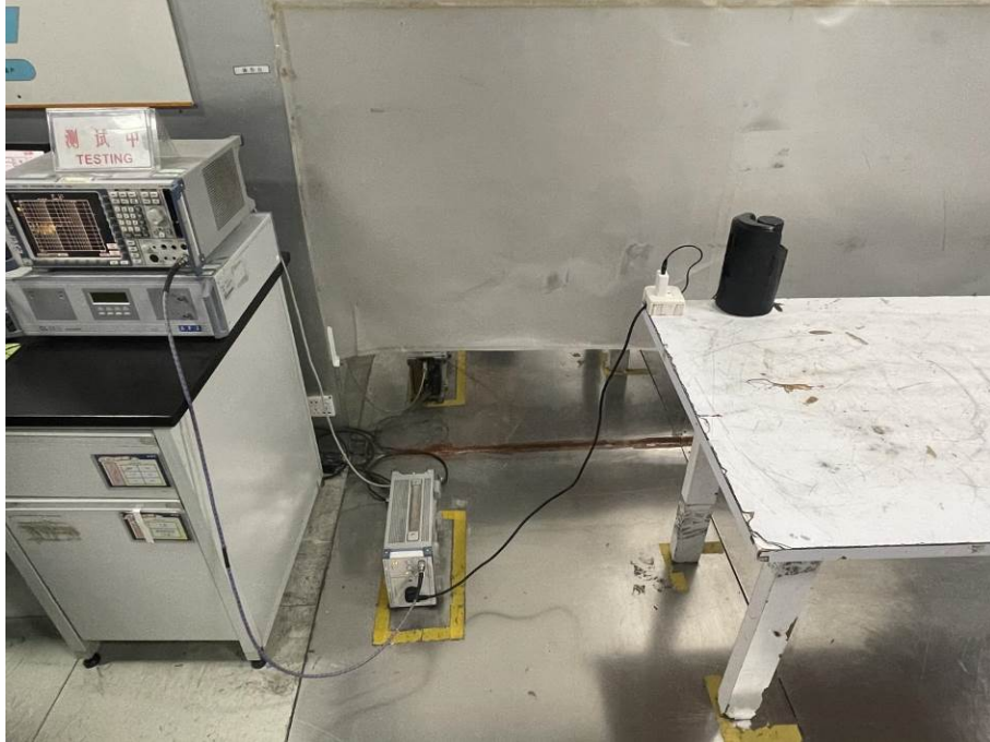
Conducted Emissions Test Setup
