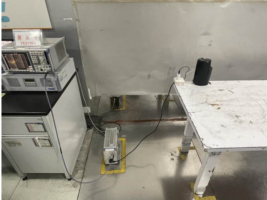
Conducted Emissions Test Setup
