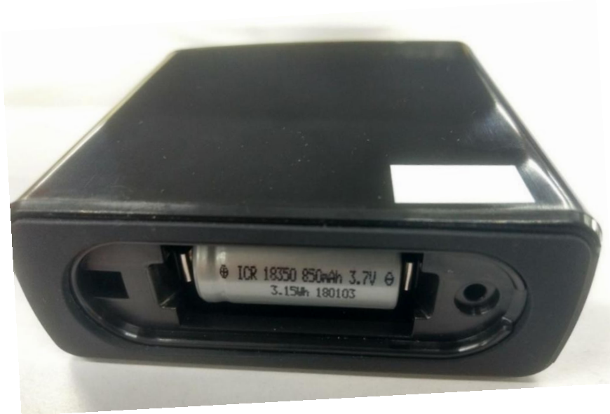
Figure 6 – Li-ion battery compartment and placement with polarity
