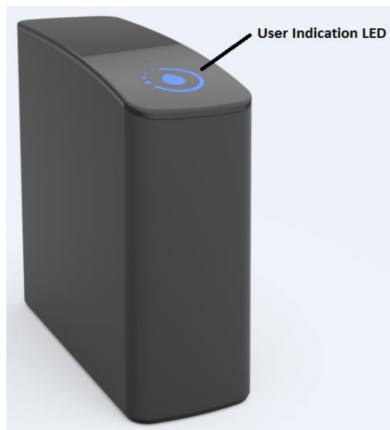
Figure 10 – Hub3.0 user interaction LED
