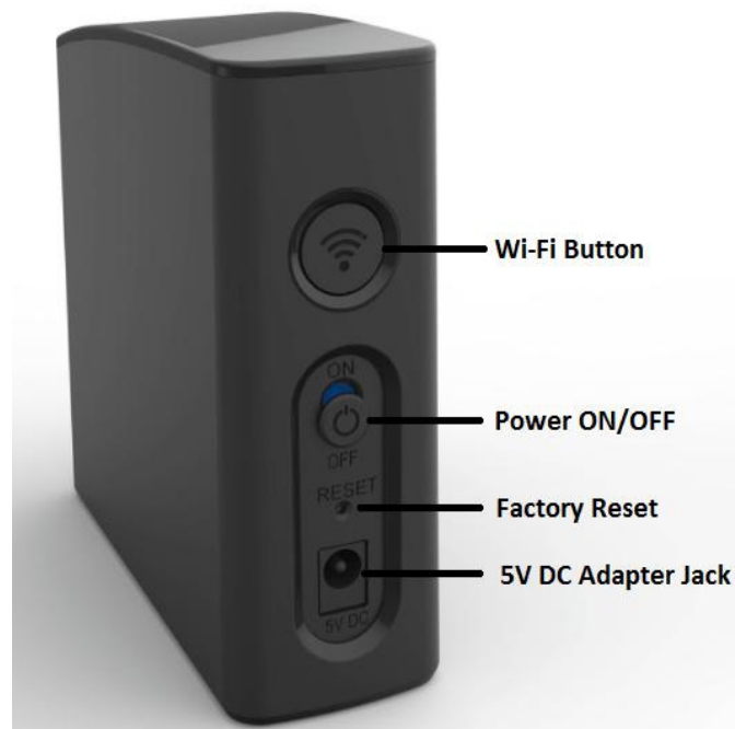
Figure 9 – Hub3.0 switch details
