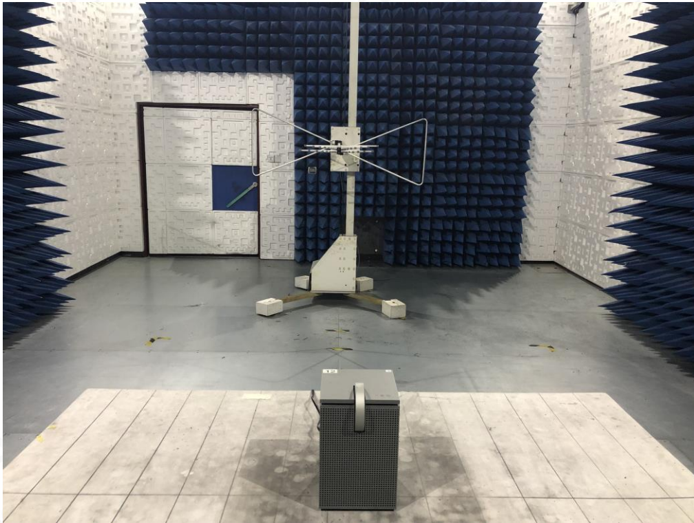
RADIATED EMISSION TEST SETUP ABOVE 1GHZ
