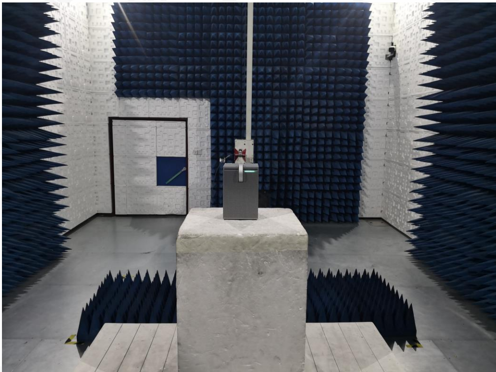
RADIATED EMISSION TEST SETUP ABOVE 1GHZ
