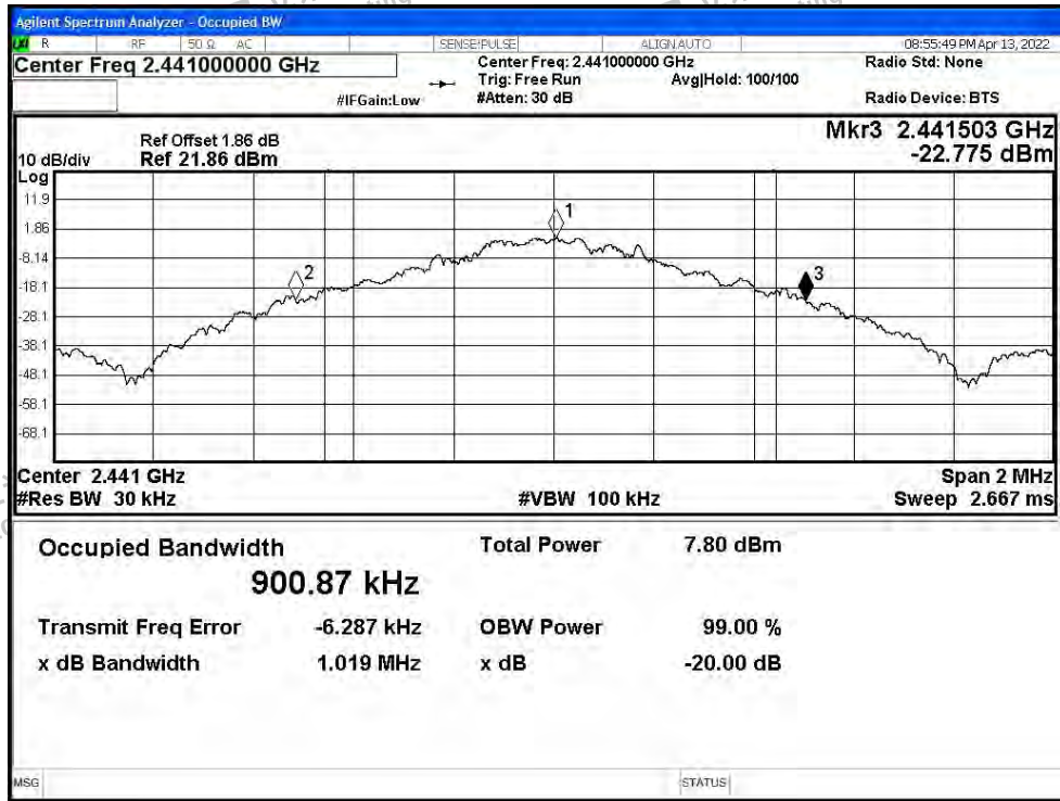
-20dB Bandwidth NVNT 1-DH5 2441MHz Ant1
