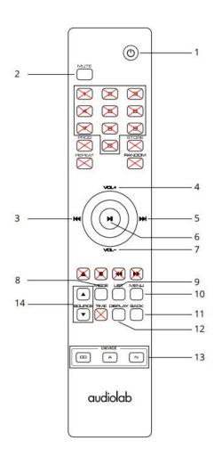
STANDBY Press to bring the unit in/out of Standby
